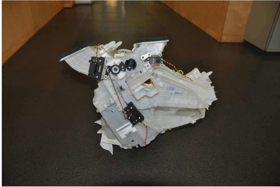
Figure 6: Photo of the HVAC-box with mounted servo motors [7]
