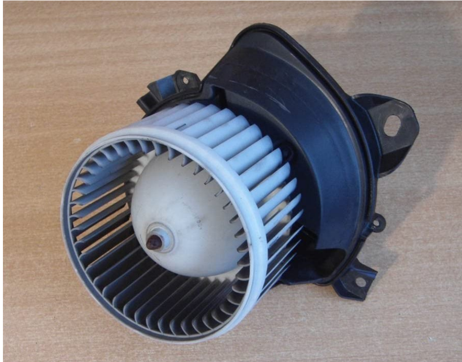
Figure 8: Photo of the blower motor.
