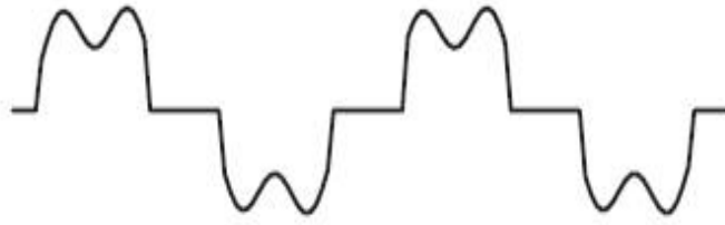
Figure 2.2 a distorted sine waveform [1]
