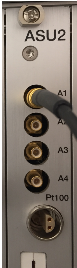
Figure A.3: Connection point of the MCR 702 to the frequency generator.
