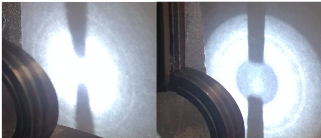
Figure 2.9: Illustration of the light distribution around the experimental area. For the visualization of the light distribution, a piece of paper was used. Left: Light distribution in long distance from the reflector position. Right: Reflector positioned very close to the measuring system. At the centre, the light intensity maximum is visible.
