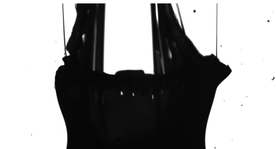
Figure 3.34: Solid behavior of PS M_w = 45,000 \text{ g} \cdot \text{mol}^{-1} at a temperature of 150 \text{ }^\circ\text{C} . The lower black rectangle represents the specimen. The upper part of the picture shows some thread formations due to sticking of the sample on the upper endplate. The sample stores the deformation energy, and no further physical deformation was observed.
