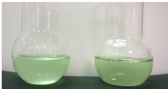
Figure 5-2 Catalyst paste dissolved in the solvent mixture 70w % n -undecane/30 w% n -octanol; left: no additional heating was used - the paste is not fully dissolved; right: additional heating at 70 °C for 1h - the paste is fully dissolved
