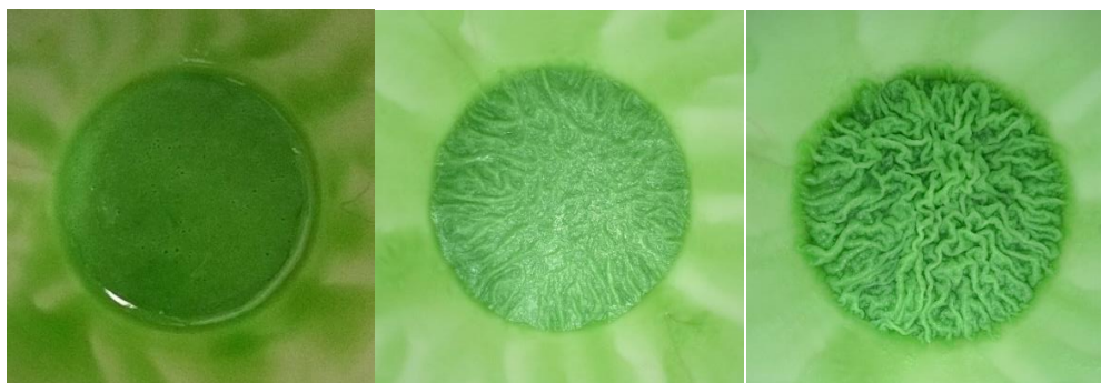
Figure 5-1 Metallosurfactant catalyst with the stoichiometric ratio of 1:2 (nickel to 4-DBSA) right after mixing (left), 40 minutes of drying (middle), and 210 minutes of drying (right)
