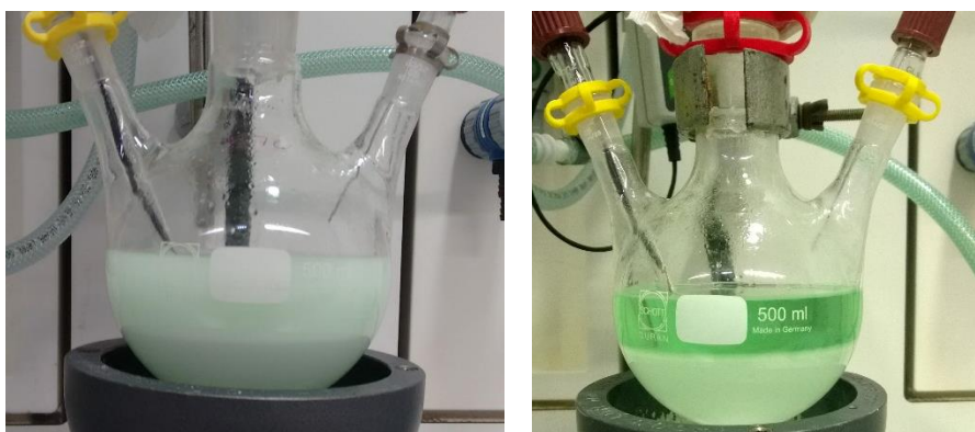
Figure 6-1 Phase separation after the esterification reaction with two different catalyst solutions . Left: SS_AT_070; right: SS_AT_015
