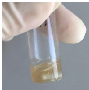
Figure 14. Picture of the OMP with 10 wt.% LiTFSI content after 24 h in the drying chamber.
