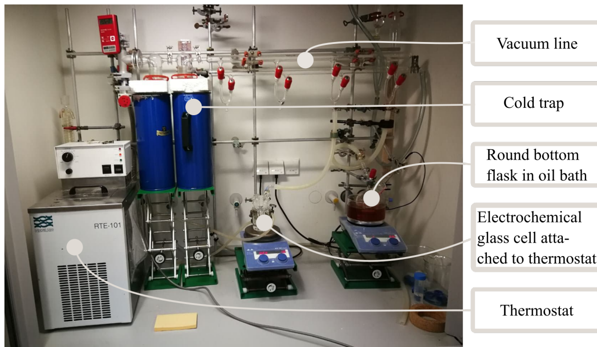
Figure 7: Picture of the setup used to dry the ionic liquid mixture. In this picture a glass cell and a round bottom flask are connected to the vacuum line. The glass cell is heated with a thermostat, the round bottom flask with an oil bath.
