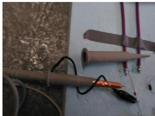
Fig. 8.9: Shielding of the probe head [2], © 2019 IEEE
