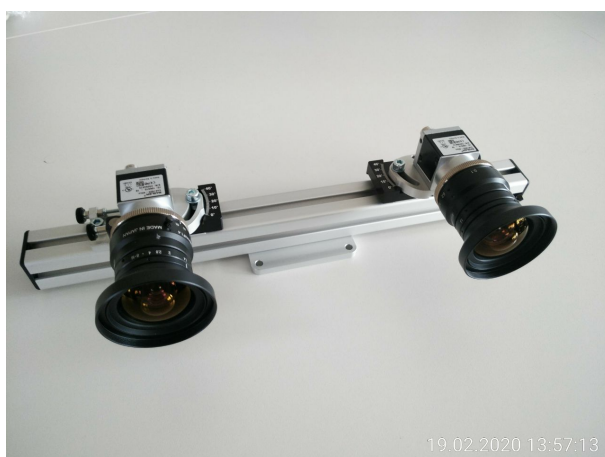
Figure 6.1: The stereo camera setup consists of two Basler acA1920-40uc cameras and an adjustable stereo rig.
