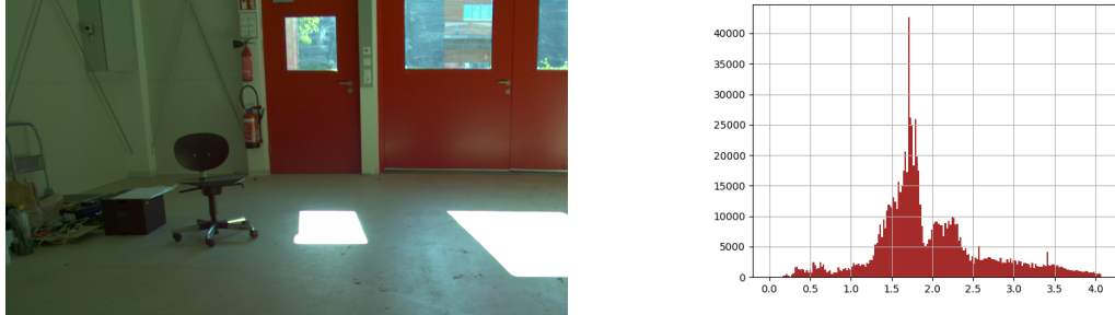
Figure 6.7: The Figure shows the example of an image and its brightness histogram when the controller has minimized the error.
