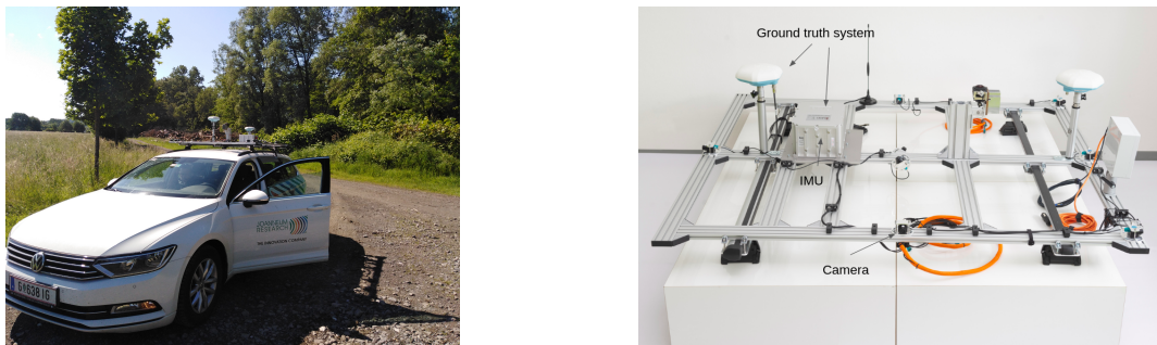
Figure 7.5: The picture on the left shows the platform used to collect the Strass dataset and on the top is the sensor plate. A general sensor setup on top plate is shown in the right picture (image credits: JOANNEUM RESEARCH).
