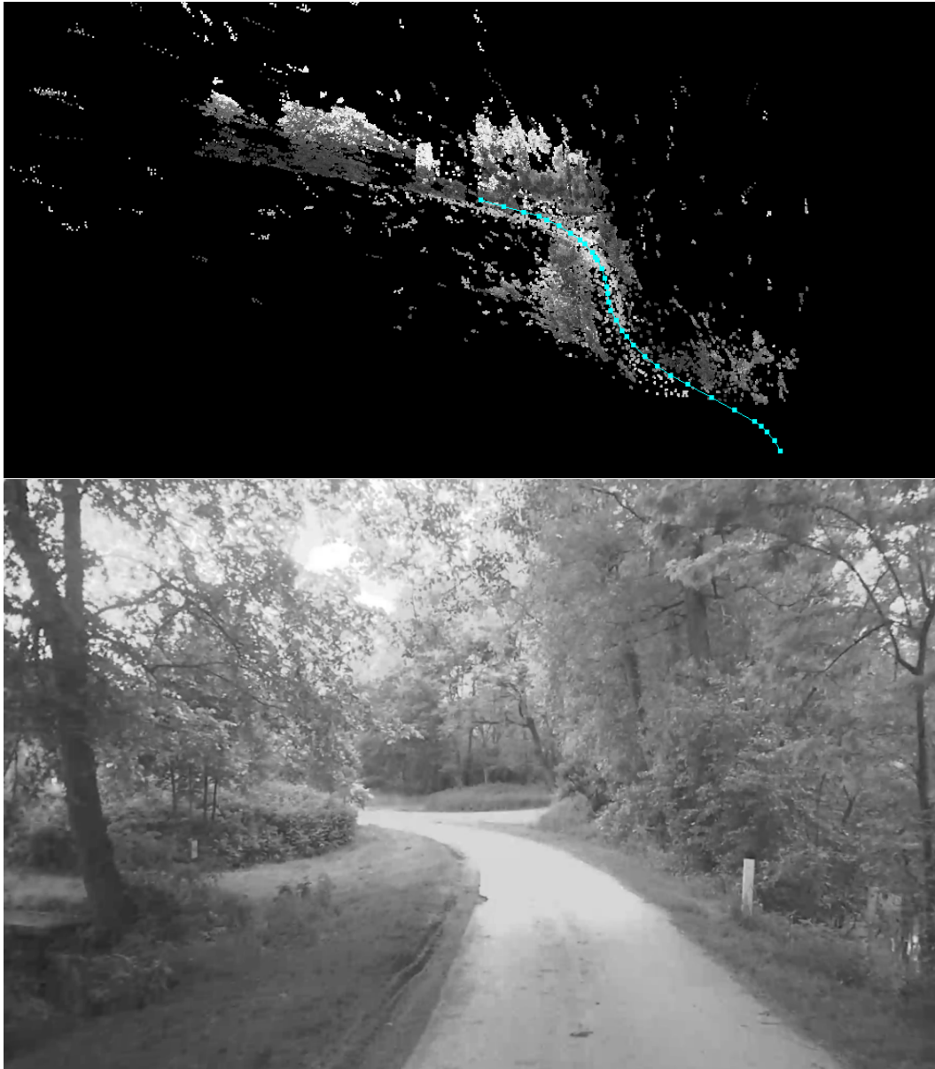
Figure 8.13: The pictures show the 3D pointcloud map (top picture) created using RTAB-Map for the Strass dataset, and a sample image (bottom picture) from the Strass dataset.
