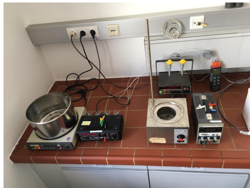
Figure 3.7.: The heat bath 3 and 4 with the corresponding Power Supplies.
