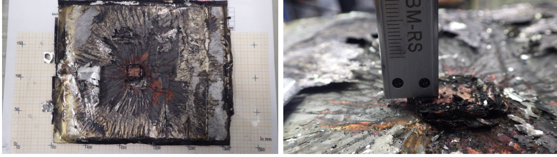
Figure 4.135: T0181. Cell after the TR experiment. Note the remaining material directly below the heat conductor. A pillar with a heights of 1 mm to 2 mm remains at the area which was directly below the heat conductor.
