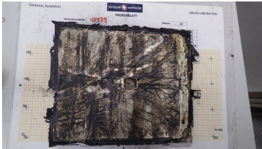
Figure 4.21: Experiment T0179, cell after TR experiment.
