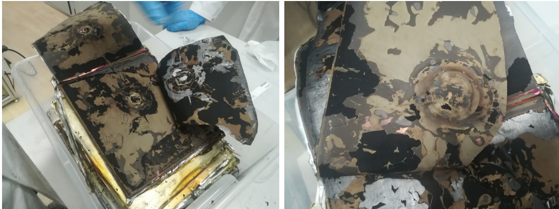
Figure 4.33: T0146a. The upper cell layers after the hot-spot experiment. The heater melted a hole through the first cathode layer (Cu current collector foil) and through the first anode layer (Al current-collector foil). Note the circular feature of the following less damaged layers.
