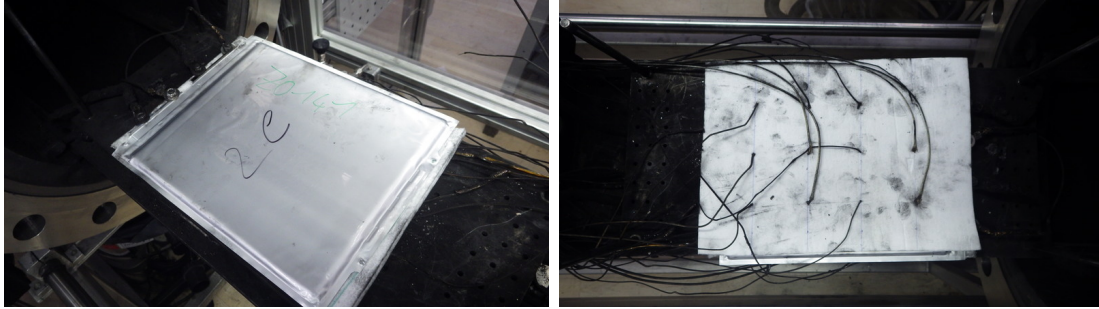
Figure 3.36: T0133. Tested cell and the thermocouple positions on the and upper side of the cell.
