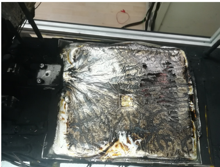
Figure 4.52: T0149. The cell after TR. Note the wrinkles that originate at the hot spot device on the tab. Note also that the cell reached its highest temperature on the remote side further away from the hot-spot. The square in the middle is only an impression from the imperfect filling of the hole for the central heater.
