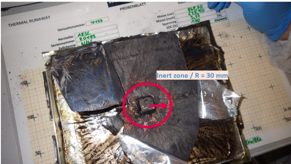
Figure 4.98: T0177. Cell after the TR experiment. In the opened cell a inert zone can is annotated in the first upper layers.
