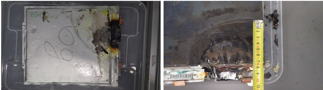
Figure 4.61: T0151. (left) Cell after the experiment. (right) details of the area near the heated tab in the dismantled cell.
