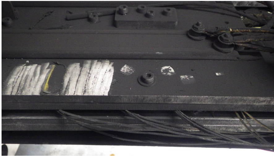
Figure 1.6: Cell holder covered with particles which were released by the cell during the venting and during thermal runaway. Particle samples were taken, where white spots are seen.
