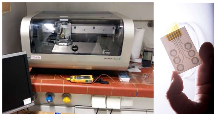
Figure 5: Left: Ink-jet printer (Fujifilm Dimatix DMP 2850). Right: printed tattoo electrodes (©Lunghammer - TU Graz).
