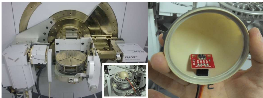
Figure 14: X-Ray diffraction goniometer with doomed heating stage equipped with a humidity sensor.
