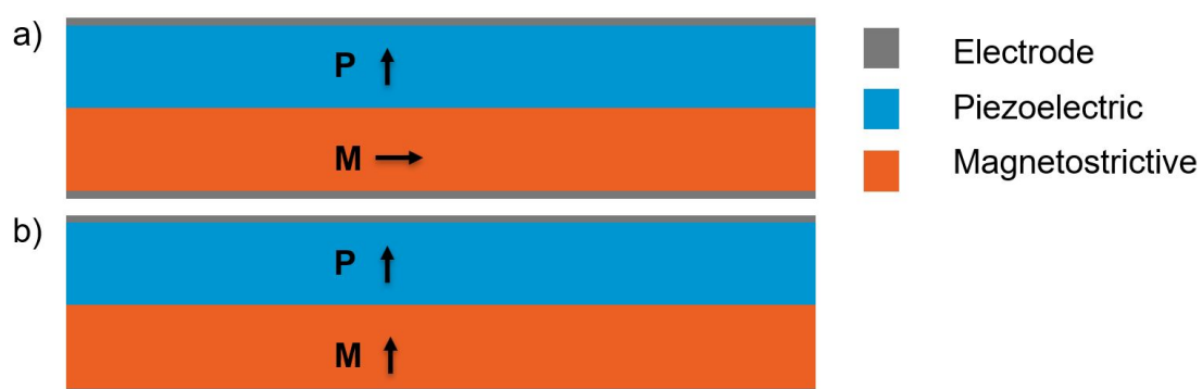
Figure 3.6: a) Transversal or in-plane and b) longitudinal or out-of-plane orientation of the magnetization M
