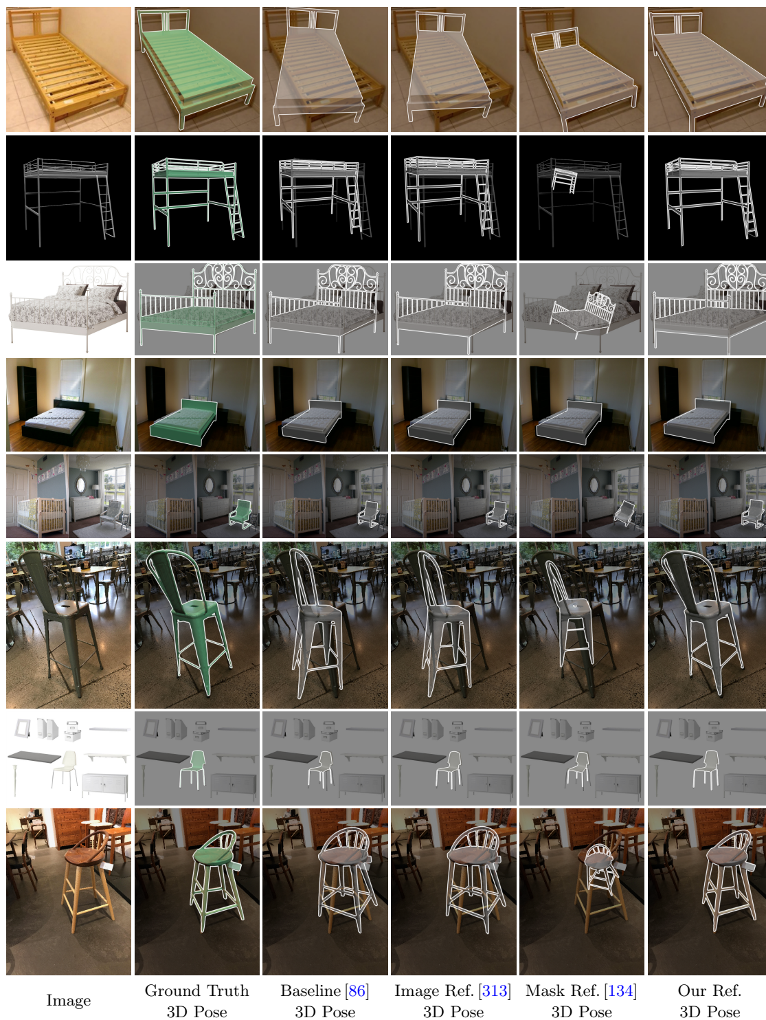
Figure 8.7: Qualitative 3D pose refinement results for objects of different categories. We project the ground truth 3D model onto the image using the 3D pose predicted by different methods. Our approach overcomes the limitations of previous methods and predicts fine-grained 3D poses which are in many cases visually indistinguishable from the ground truth.
