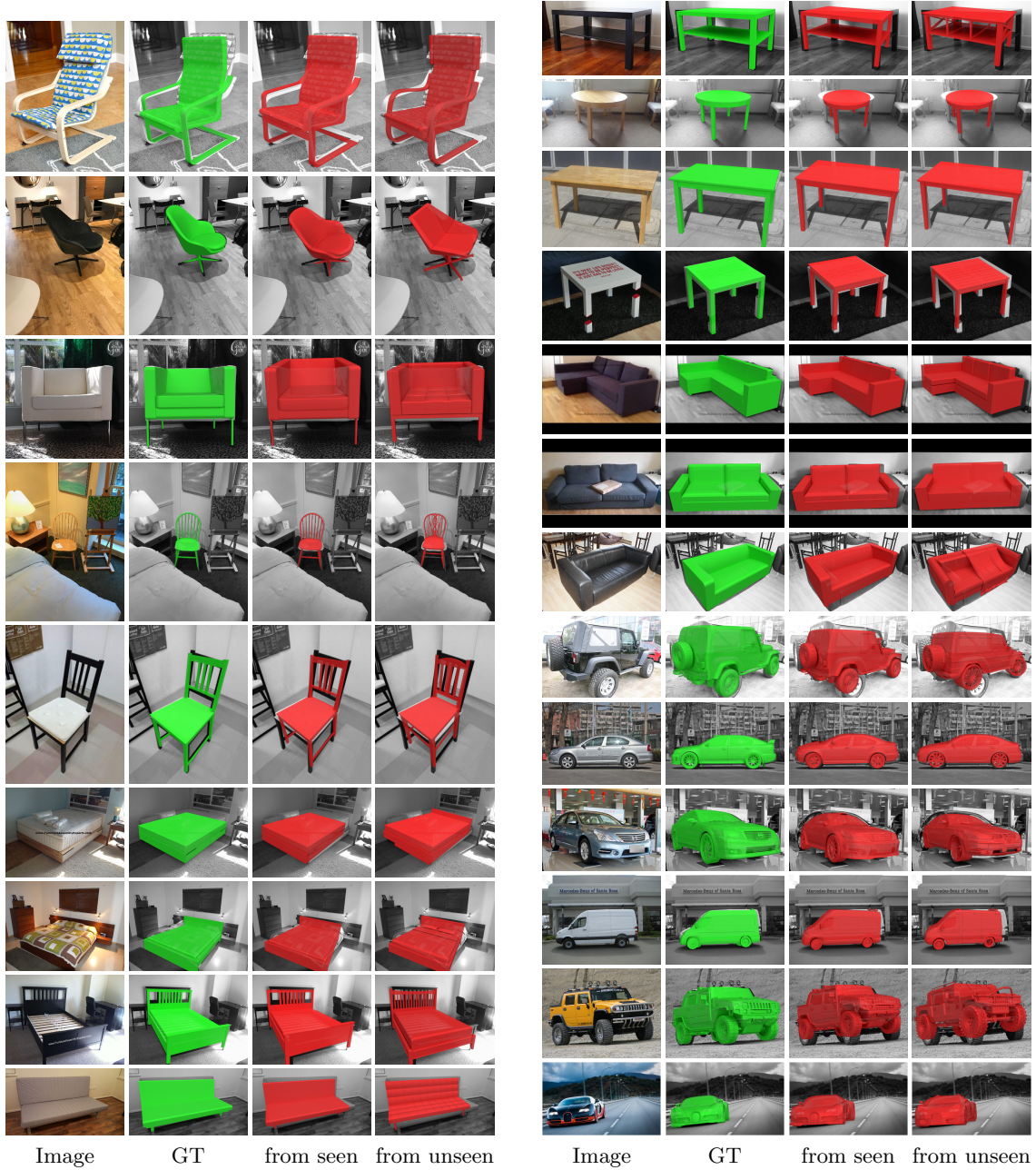
Figure 7.6: Qualitative results for 3D pose estimation and 3D model retrieval from both seen and unseen databases. We project the retrieved 3D model onto the image using a 3D pose computed from the predicted location field by solving a PnP problem. For the ground truth 3D model, we use the ground truth 3D pose. In fact, location fields provide all relevant information to jointly address both tasks.
