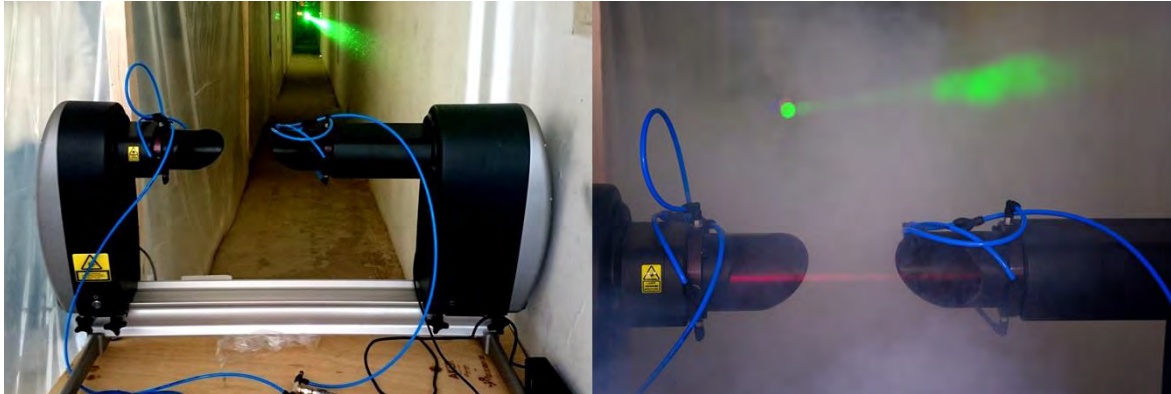
Figure 5.10: Spraytec Malvern device for PSD analysis installed in the middle of 50 m Koruza fog channel (The figure is partly obtained from own publication [83])
