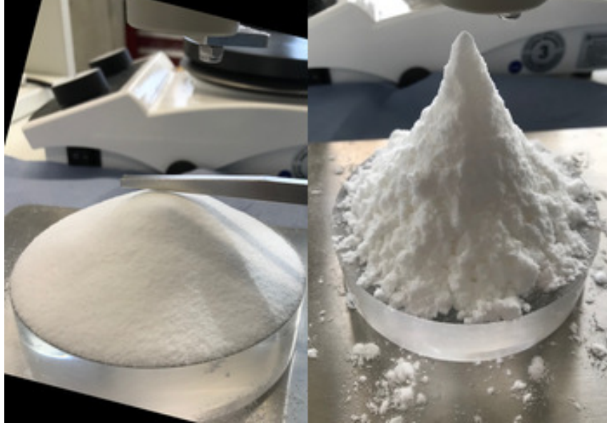
Figure 4.8: Pictures of the AoR testing phase for LAC (left) and ASA (right). The high cohesiveness of the latter makes its slope steep and craggy, especially when compared to the broad smooth surface of the LAC pile.
