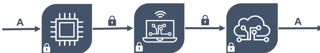
Figure 4.19: Communication participants for end-to-end secured communication. Edge nodes send encrypted messages to a gateway that forwards the data to a virtual kiosk unit for further processing
