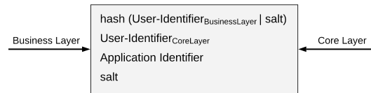
Figure 4. Privacy preserving mapping of a user object between business layer and core layer – confidential data remains on the business level.
