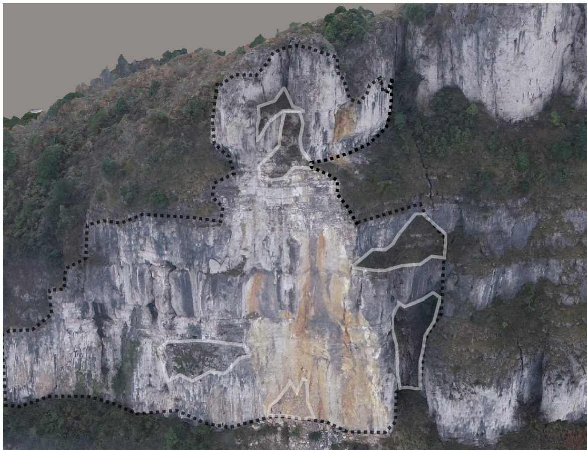
Figure 4-2: Delineation of "Rockfall Area". Regions with vegetation cover obscuring the rock surface have been excluded from the analysis, and are outlined in white.
