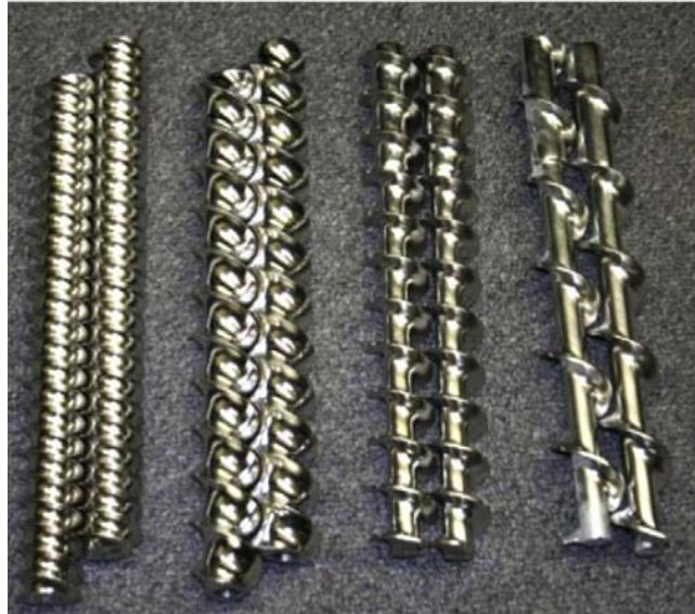
Figure 6: Twin-screw model: fine concave screw, coarse concave screw, fine auger screw, and coarse auger screw. [21]
