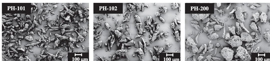
Figure 11: MCC particle shape and size distribution for different grades[33]
