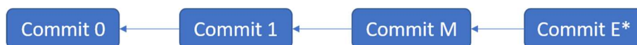
Figure 5: The rebasing process results in a much cleaner commit history but the snapshot of the merging (“Commit E”) and rebasing results (“Commit E*”) are the same.
