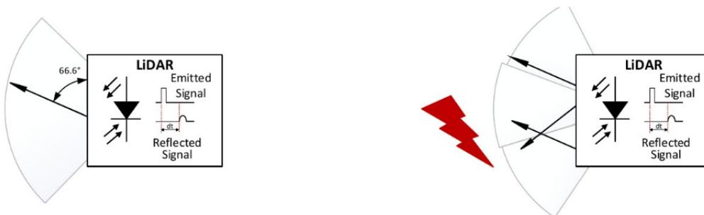
**Figure 4.9:** Interference between several LiDAR systems caused by the circumstance that the lasers are crossing each others.
