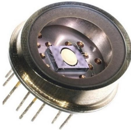
**Figure 3.21:** MEMS mirror of the 1D MEMS Micro-Scanning LiDAR platform [3].
