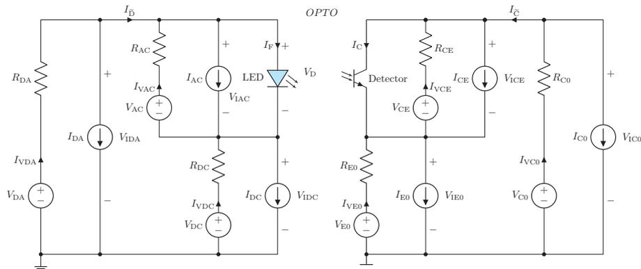
Figure B.9: Optocoupler Circuit-Model with I/O interface.
