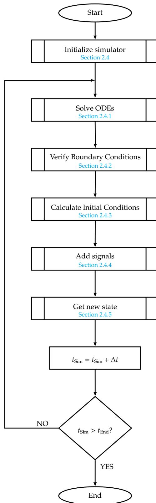
Figure 2.6: Flowchart for transient analysis.
