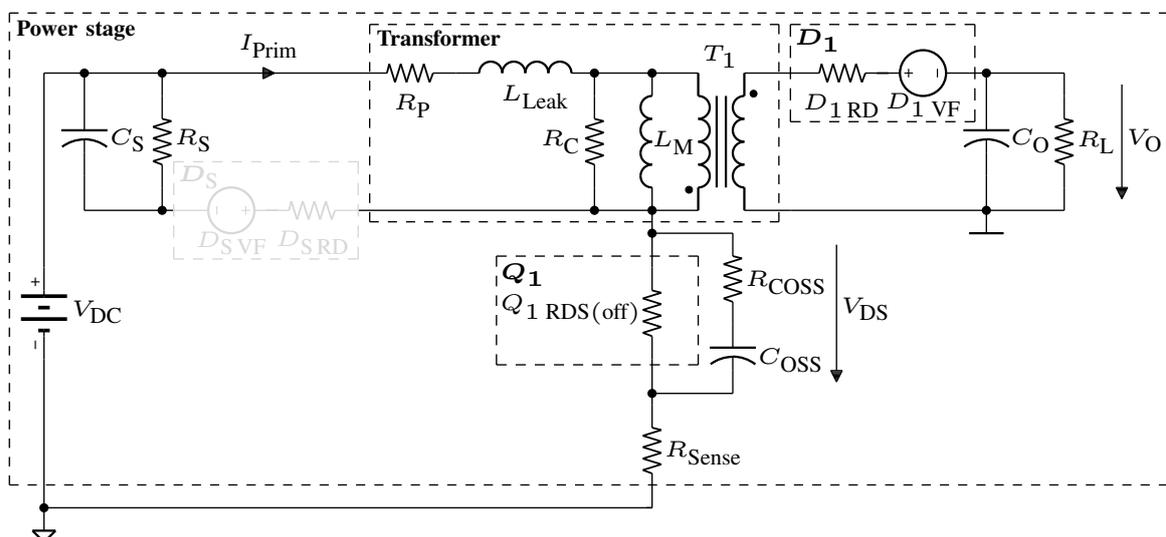
Figure 3.6: Open-loop flyback converter SubCircuit-Model III.
