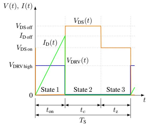
Figure 5.6: Simulated MOSFET switching waveforms for one switching period  $T_S$  in DCM.<sup>4</sup>
