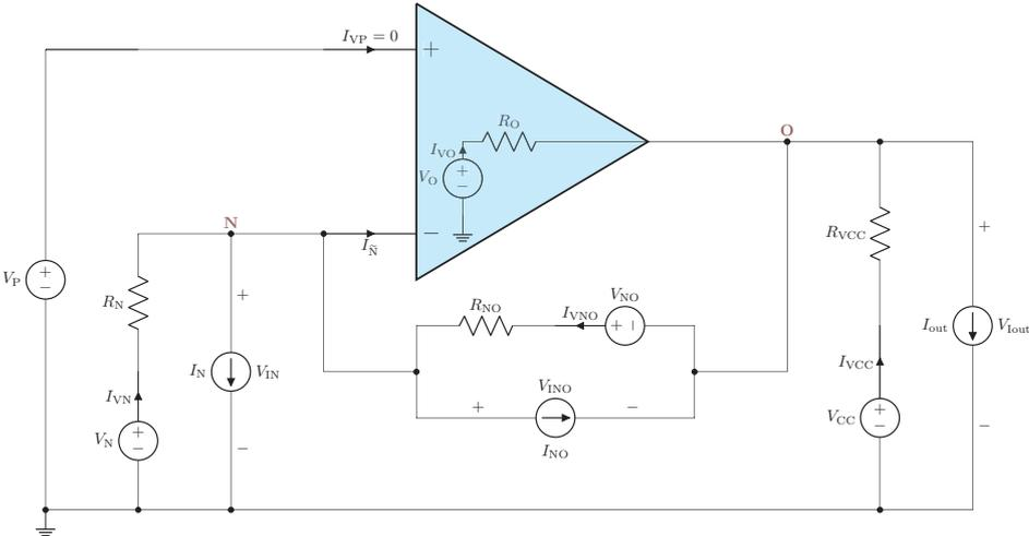
Figure B.12: Universally applicable amplifier SubCircuit-Model.
