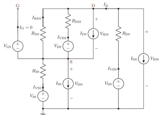
Figure B.5: Universally applicable MOSFET SubCircuit-Model.
