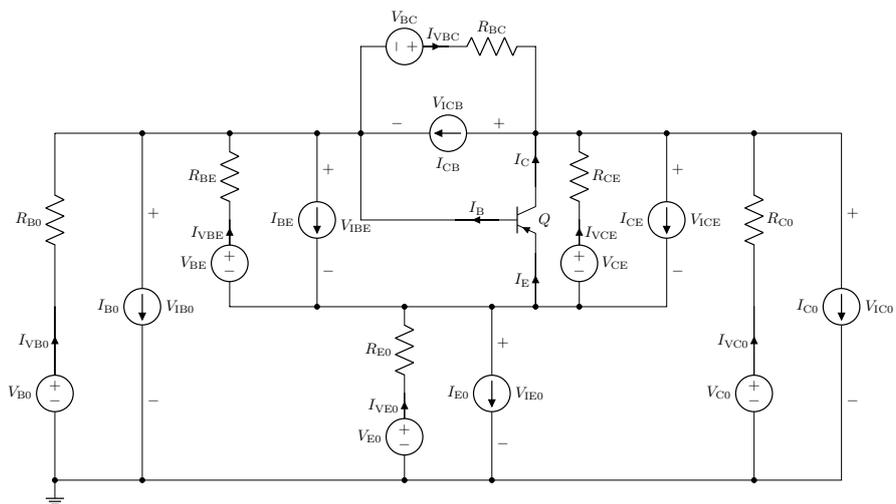
Figure B.7: PNP BJT Circuit-Model with I/O interface.
