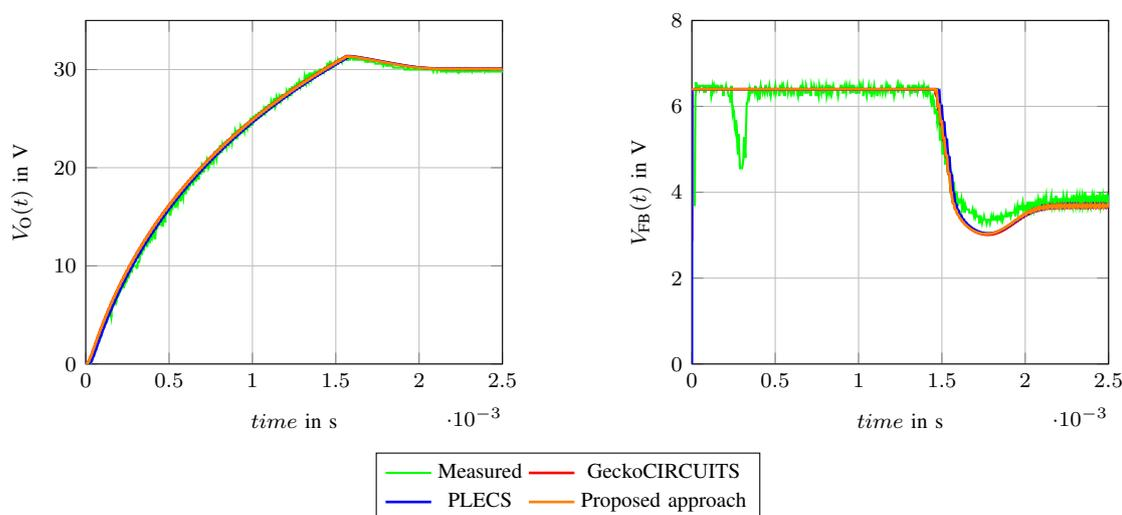
Figure 3.9: Comparison of measurement and simulation results:  $V_O(t)$  and  $V_{FB}(t)$  closed-loop flyback converter during start-up.
