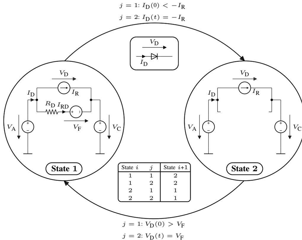
Figure 2.5: Diode state diagram.
