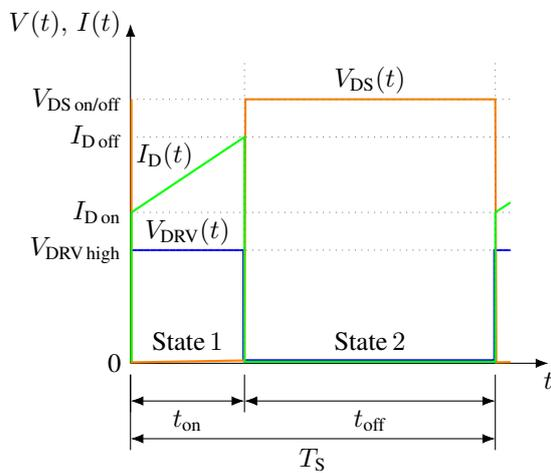
Figure 5.5: Simulated MOSFET switching waveforms for one switching period  $T_S$  in CCM.
