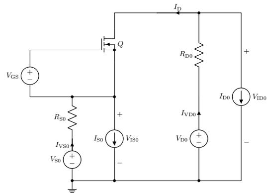
Figure B.3: N-channel MOSFET Circuit-Model with I/O interface.
