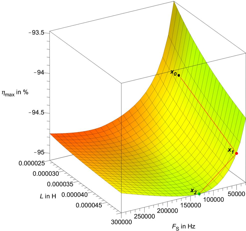
Figure 5.7: Step down converter  $\eta_{\max}(F_S, L)$ .
