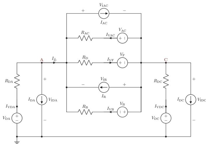
Figure B.2: Universally applicable diode SubCircuit-Model.
