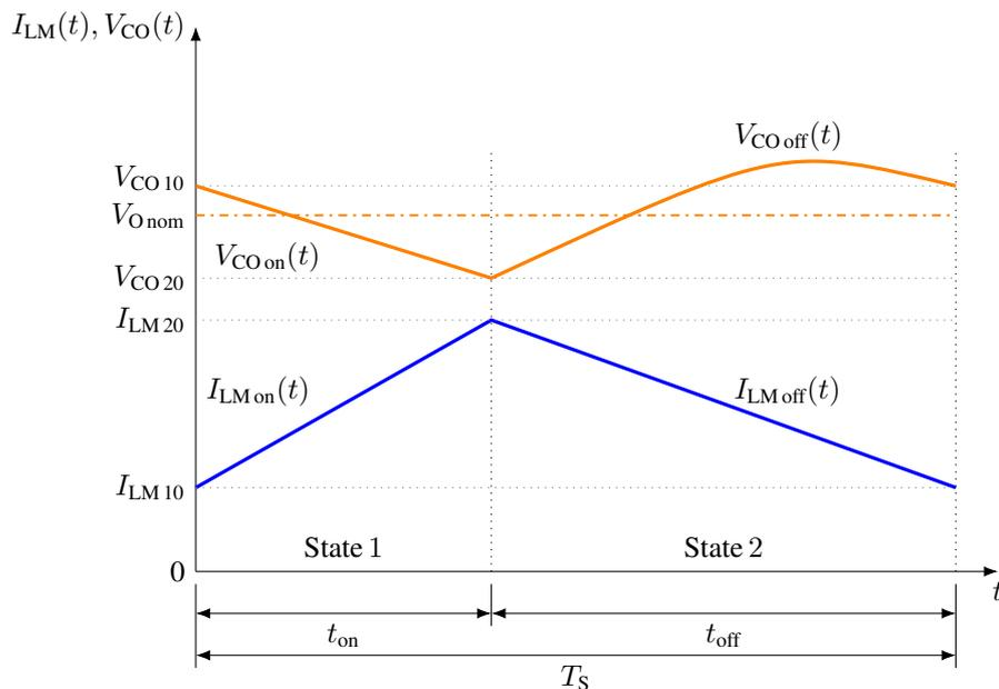
Figure 4.6: Waveforms flyback.
