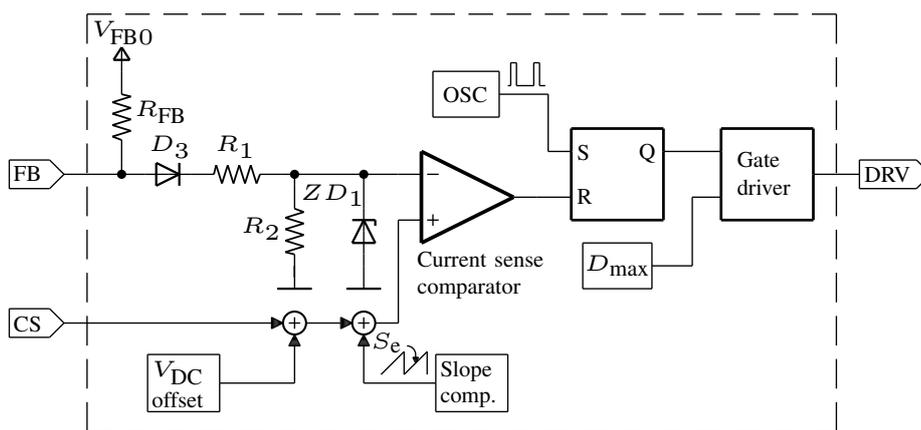
Figure 3.3: Block diagram of the peak current mode PWM controller.
