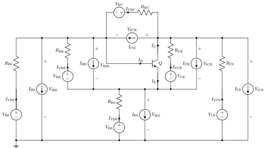
Figure B.6: NPN BJT Circuit-Model with I/O interface.
