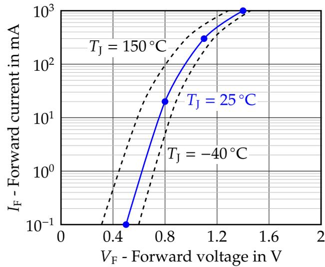
Figure 1.1: Illustrated forward voltage characteristic for different junction temperatures  $T_J$  of a GP diode.
