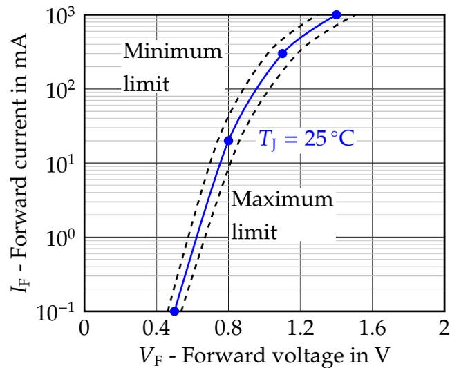
Figure 1.2: Illustrated forward voltage characteristics with limits of a GP diode.
