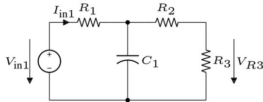
Figure 2.4: Interconnected SubCircuit-Model, connecting the SubCircuit-Models shown in Figure 2.1 and Figure 2.2.
