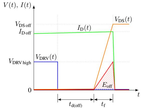
Figure 5.4: Simulated MOSFET switching waveforms during turn-off.
