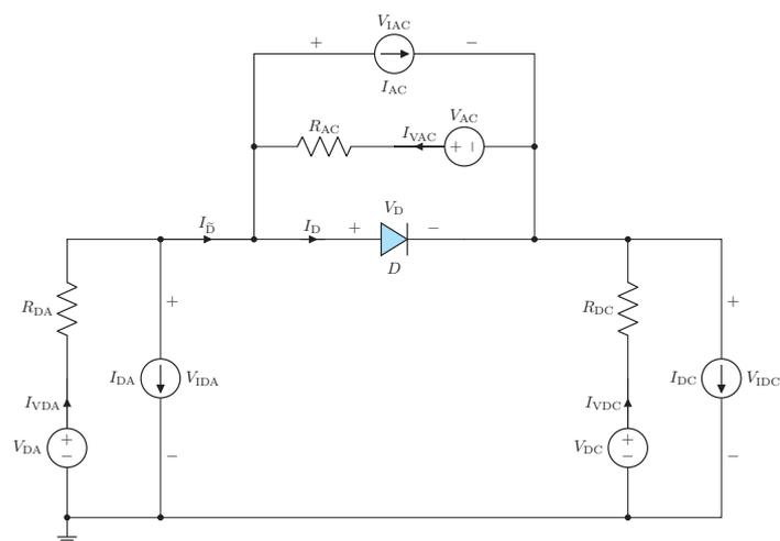
Figure B.1: Diode Circuit-Model with I/O interface.
