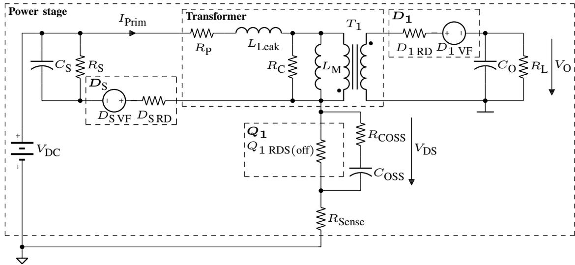
Figure 3.7: Open-loop flyback converter SubCircuit-Model IV.
