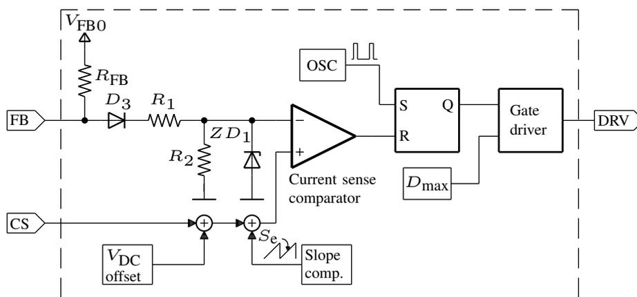
Figure 4.5: Block diagram of the peak current mode PWM controller.
