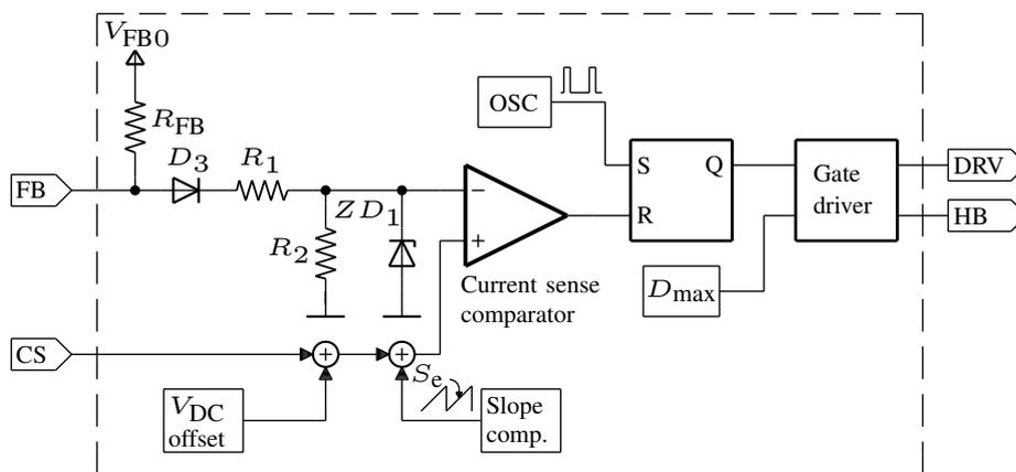
Figure 5.2: Block diagram of the peak current mode PWM controller.
