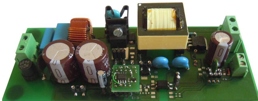
Figure 3.1: Flyback converter prototype.
