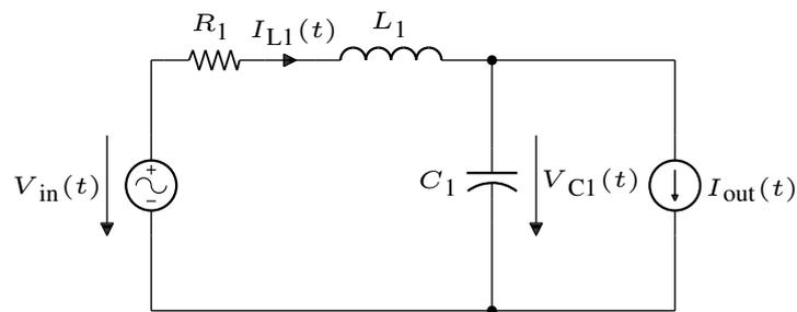
Figure 4.1: SubCircuit-Model: RLC series resonant circuit.
