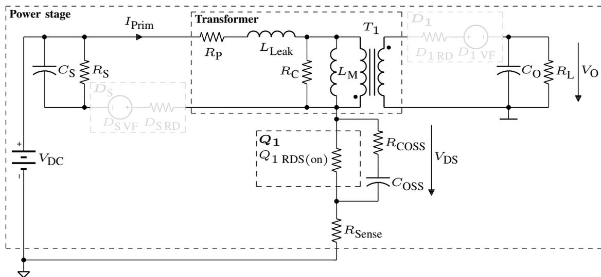
Figure 3.4: Open-loop flyback converter SubCircuit-Model I.
