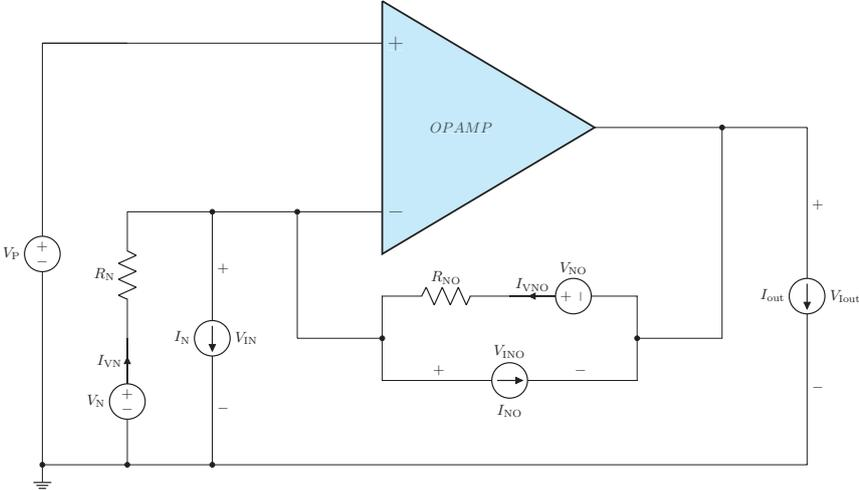
Figure B.11: Amplifier Circuit-Model with I/O interface.
