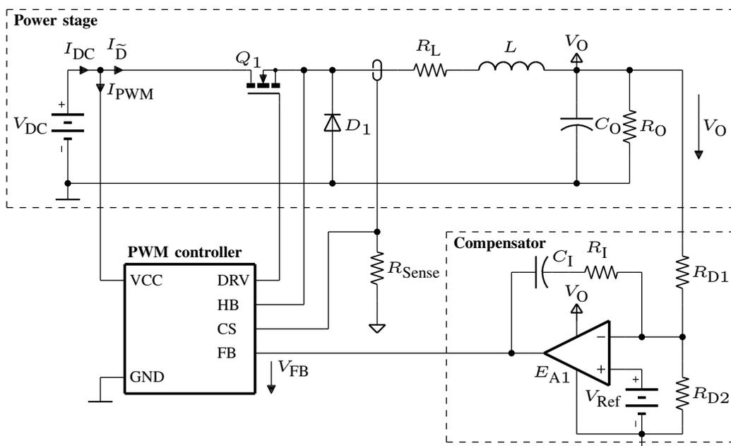
Figure 5.1: Schematic diagram of a closed-loop step down converter with peak current mode control.
