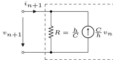
Figure 1.4: Discrete circuit models for a linear capacitor, [11].
