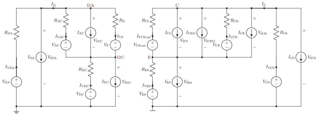
Figure B.10: Universally applicable Optocoupler SubCircuit-Model.
