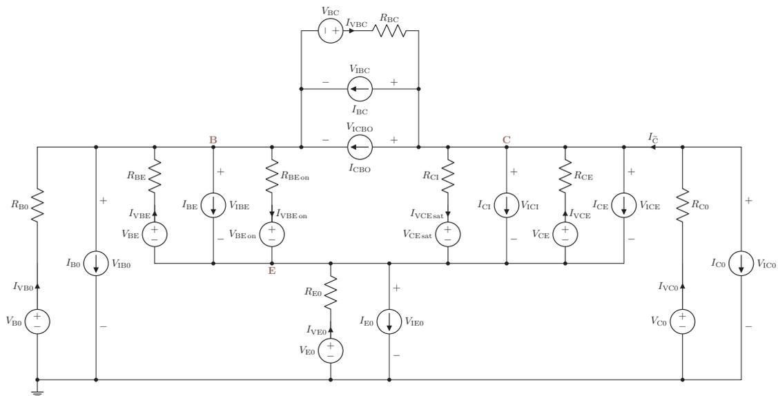
Figure B.8: Universally applicable BJT SubCircuit-Model.
