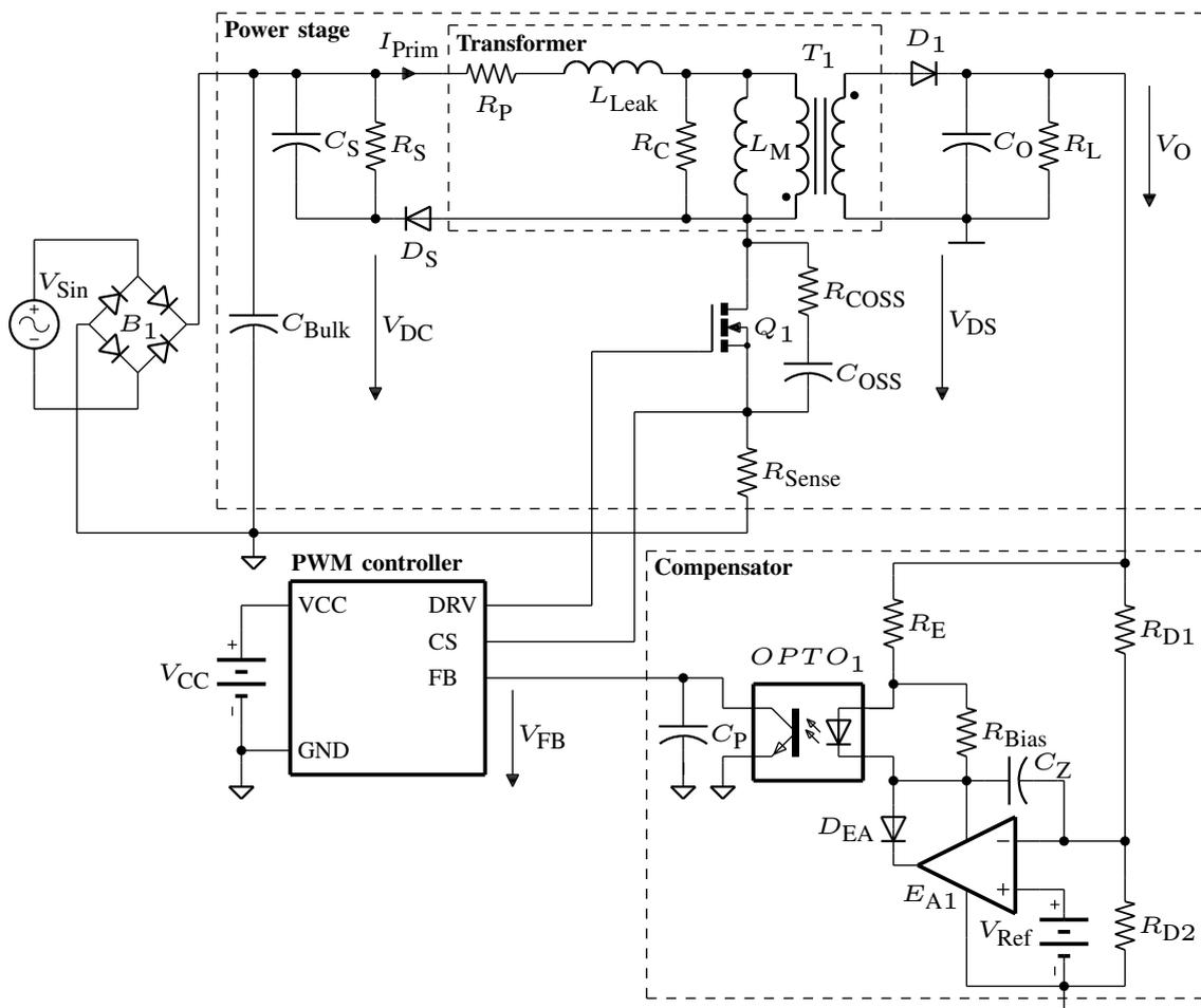
Figure 3.2: Schematic diagram of a closed-loop flyback converter with peak current mode control.
