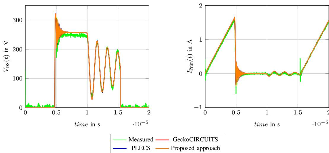
Figure 3.8: Comparison of measurement and simulation results:  $V_{DS}(t)$  and  $I_{Prim}(t)$  open-loop flyback converter in steady-state.
