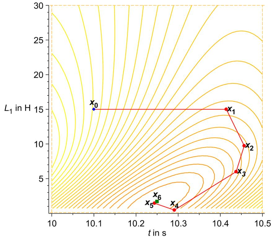
Figure 4.3: RLC series resonant circuit contour plot  $I_{L1 \max} \text{function}(t, L_1)$ .
