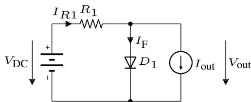
Figure 1.3: Simple voltage reference circuit.
