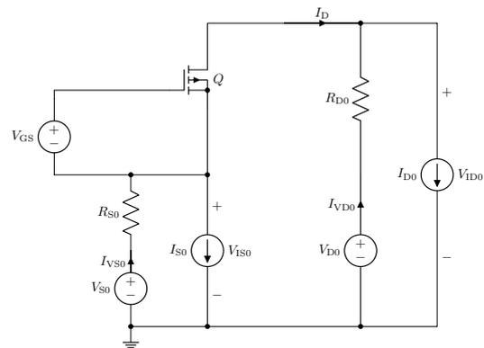
Figure B.4: P-channel MOSFET Circuit-Model with I/O interface.
