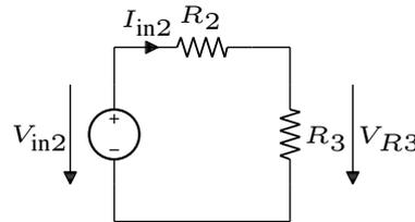
Figure 2.2: SubCircuit-Model: simple voltage divider.
