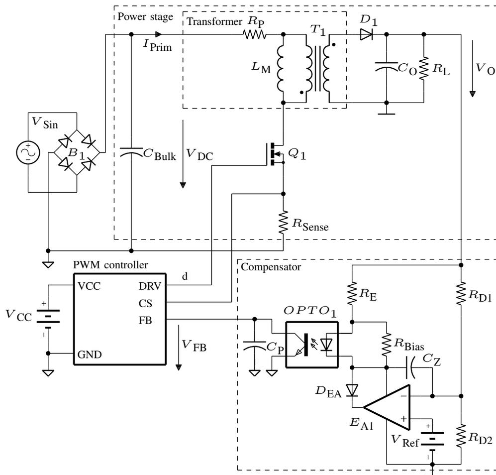
Figure 4.4: Schematic diagram of a closed-loop flyback converter with peak current mode control.
