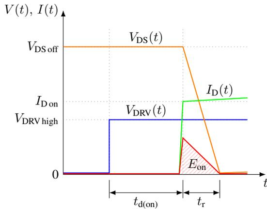
Figure 5.3: Simulated MOSFET switching waveforms during turn-on.
