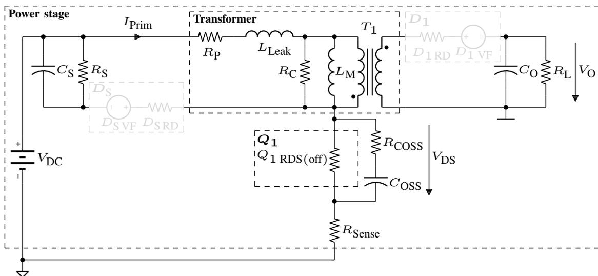
Figure 3.5: Open-loop flyback converter SubCircuit-Model II.
