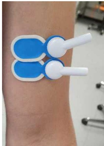
Figure 40: Electrode positioning of the adhesive EMG-electrode for the biosignal verification
