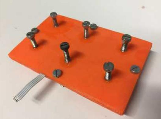
Figure 22: 3D-printed die casting mold
