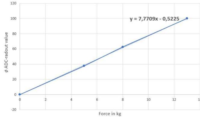
Figure 31: Relation between the average of the measured ADC value and the force, produced by the hung up weight
