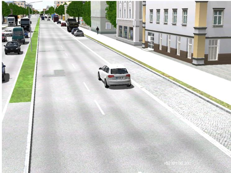
Figure 3.4: Scenario urban: Mid of scenario: The ego vehicle drives still with around 50 km/h on the right lane. After around 20 s, the ego vehicle comes to a congestion caused by a red traffic light and has to decelerate.
