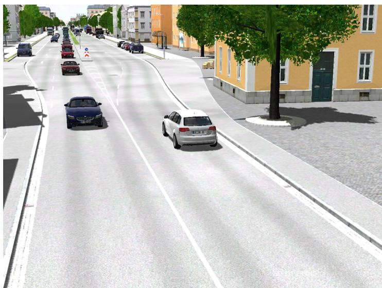
Figure 3.3: Scenario urban: Begin of scenario: The white car is the ego vehicle and drives constantly with around 50 km/h on a one-lane road with oncoming traffic. After a few seconds, the road broadens to two lanes and the ego vehicle drives on the right lane. Additionally, there are stationary vehicles parking on the right side.
