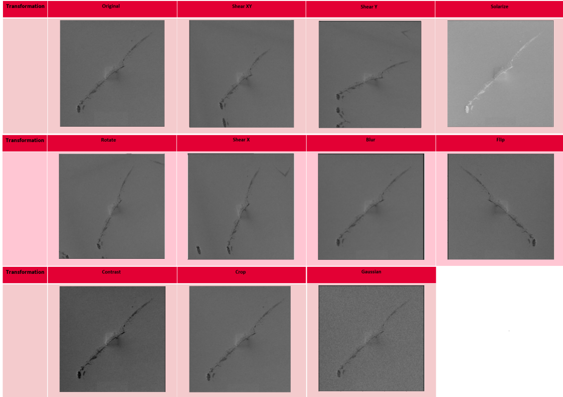
Figure 3.5: Table of image transformations. Border reflection leads to duplication of the defect for those samples where the defect is close to the border. Whether this has or not a negative effect on model performance remains to be seen.
