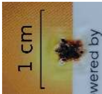
Figure 3.41: Picture showing thermal degradation of an NFC card
