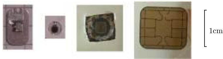
Figure 3.45: Comparison of different NFC Chips for cards
