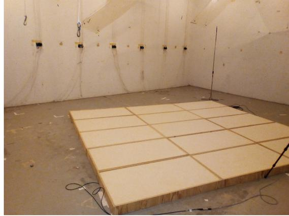
Figure 3.1: Porous absorber placed on the floor in the reverberation chamber ( $V = 241 \text{ m}^3$ ), absorber with sides covered by a wooden frame and a total area of  $S = 10.8 \text{ m}^2$
