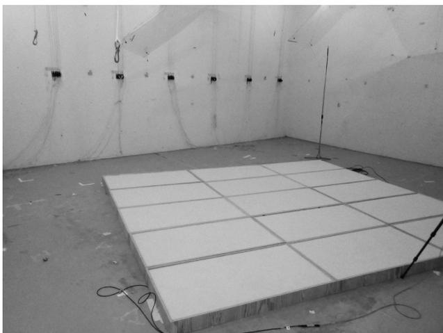
FIG. 2. Porous absorber placed on the floor in the reverberation chamber ( $V = 241$  m<sup>3</sup>), absorber with sides covered by a wooden frame and a total area of  $S = 10.8$  m<sup>2</sup>.
