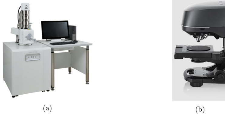
Figure 20: Pictures of the JOEL scanning electron microscope (a, SEM, Source [12]) and the Keyence laser scanning microscope (b, LSM, Source [3]).
