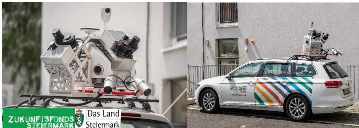
**Abbildung 5** - *Leica Pegasus: Two Ultimate Dualhead* (Foto: © Bergmann, 2018)
