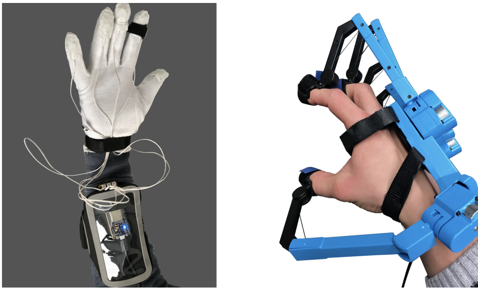
Figure 2.4.: Custom glove with vibrotactile stimulations on the left and Sense Glove DK1 on the right, used for comparison of different haptic feedback stimulations in Kreimeier et al. (2019)
