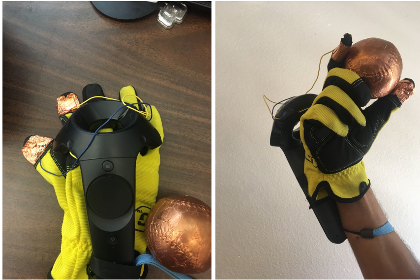
Figure 3.6.: On the left is the empty glove controller that was used during testing. On the right is an example how the baseball is held and sending a signal to the simulation.
