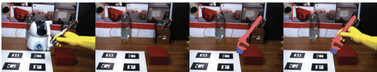
Figure 2.5.: Pipeline of visiohaptic implementation in Cosco, Garre, Bruno, Muzzupappa, and Otaduy (2012). From left to right: (a) Real world scene; (b) Virtual view after image-based removal of hand and tool; (c) Composition of virtual object; (d) Final view, free of tool-hand misalignments.
