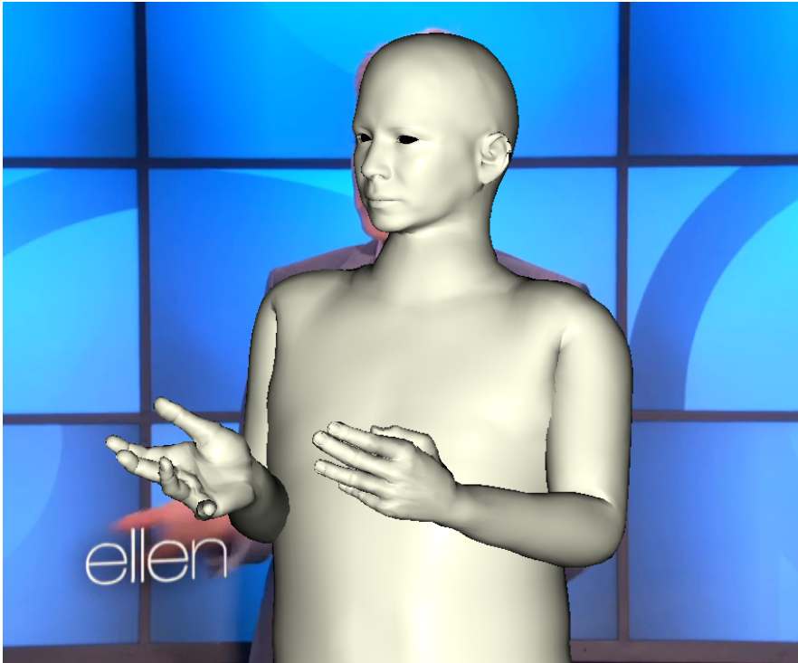
Figure 2.7.: Human Pose and Shape Estimation MTC. The model proposed by Xiang, Joo, and Sheikh (2019) shows superior accuracy compared to previous approaches on the data of Ellen DeGeneres. However, the algorithm shows still inaccuracies when estimating the 3D hand pose.
