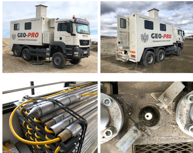
Figure 3.26: Cone penetration test with pore water pressure measurement - device
