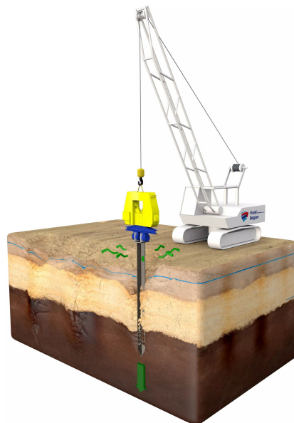
Figure 2.5: Resonance compaction method according to [3]
