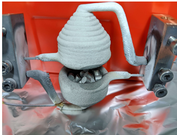
Figure C.1: Magnesium pellets in the ceramic pot, which is resistively heated inside the pickup chamber.
