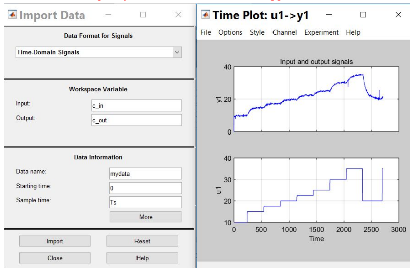
(b) Step 2: Import (left) and time-plot (right) of experimentally collected input- and output sequences
