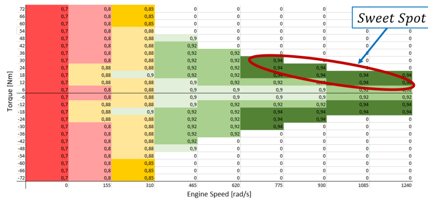
Figure 3.9.: Ibex motor efficiency map
