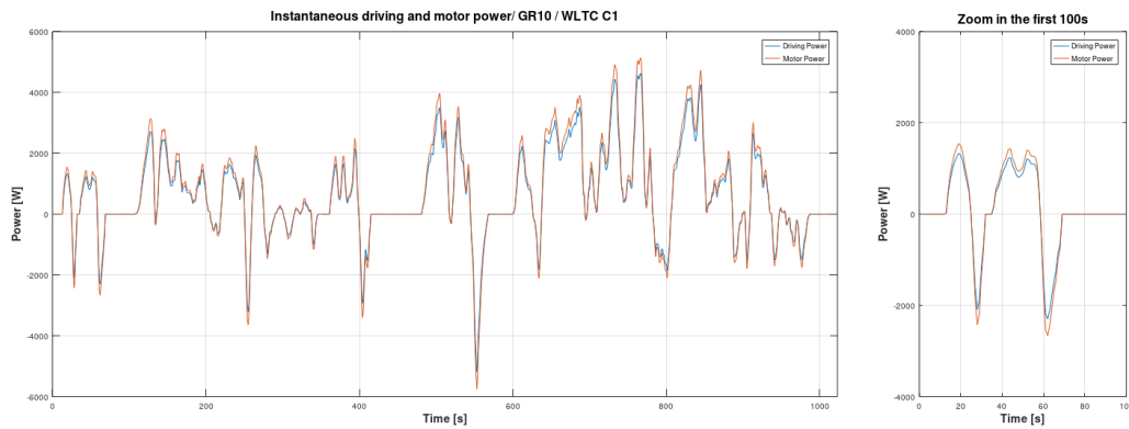
Figure 3.14.: Driving and motor power with GR=10 / WLTC C1
