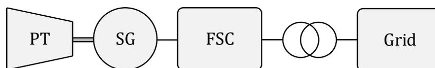
**Figure 2.7:** Block diagram of full-size converter operation of a synchronous generator in a PSPP (PT = Pump-Turbine, SG = Synchronous Motor-Generator, and FSC = Full-Size Converter).
