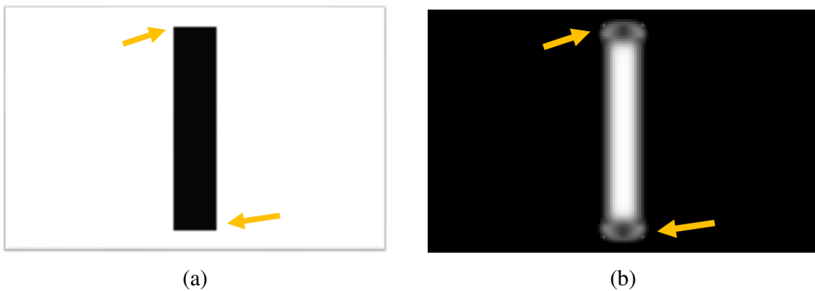
Figure 2.18 Problematic regions where tubularity assumption is not fulfilled are marked by yellow arrows presented on a slice of the “perfect tube” (Figure 2.18a) and its Frangi response (Figure 2.18b).
