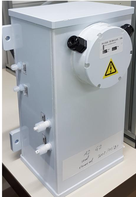
Figure 2.5.: The flow heater
