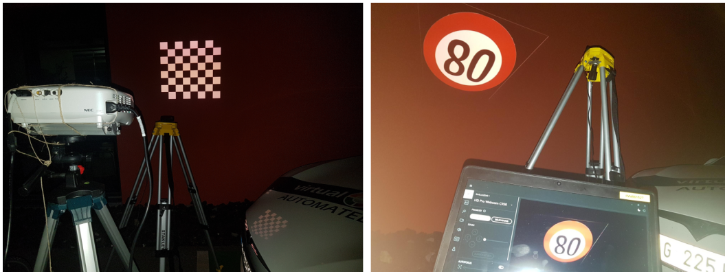
Figure 4.7: The test environment with one projector and a web-camera
