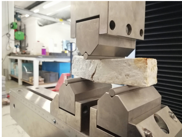
Fig. 137: MM-CS1-FS-PO-01 - at breaking point
