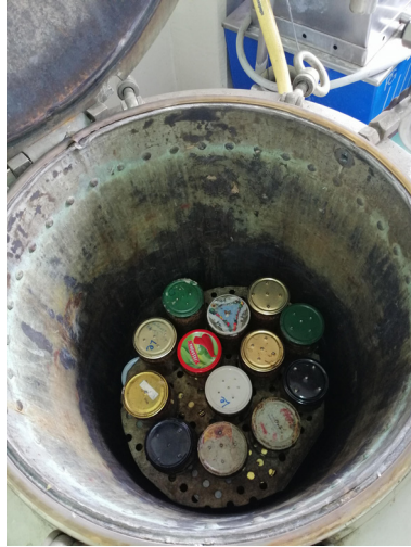
Fig. 69: Placing the substrate before sterilization
