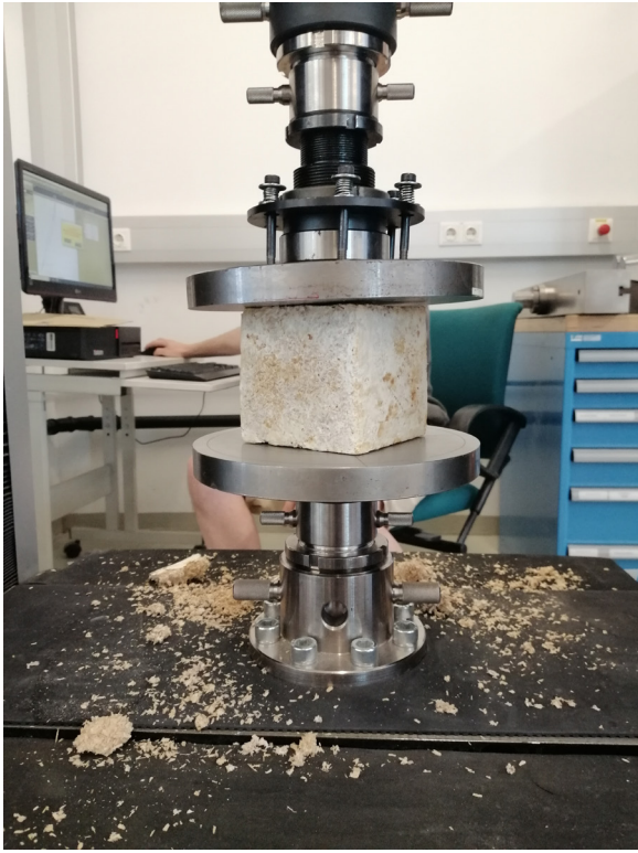
Fig. 118: Compression strength testing - before
