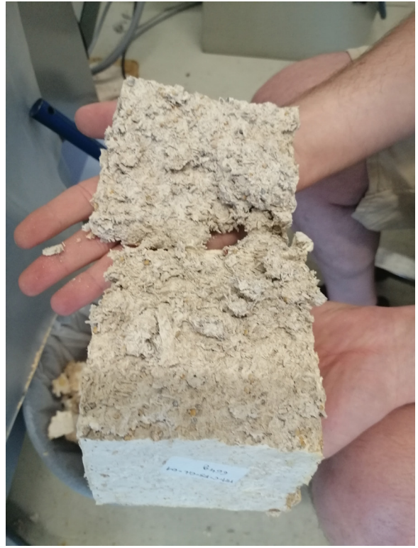
Fig. 124: After breaking - section evaluation
