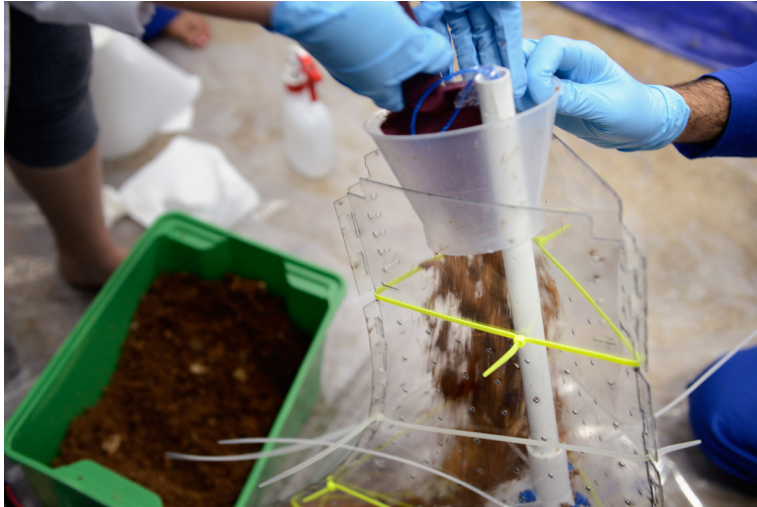
Fig. 38: Filling of the digitally fabricated moulds with inoculated substrate
