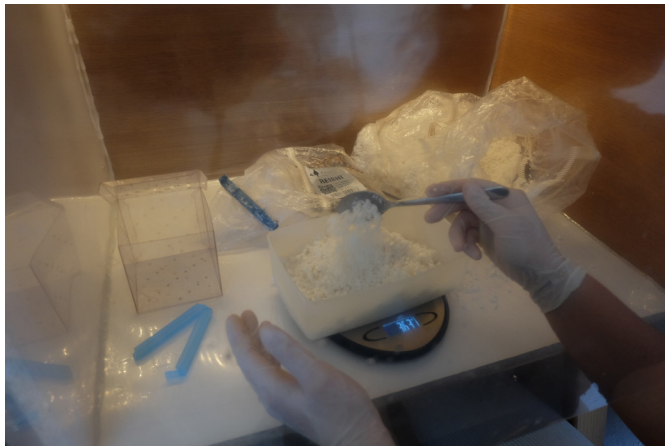
Fig. 62: Weighing the sterilized substrate
