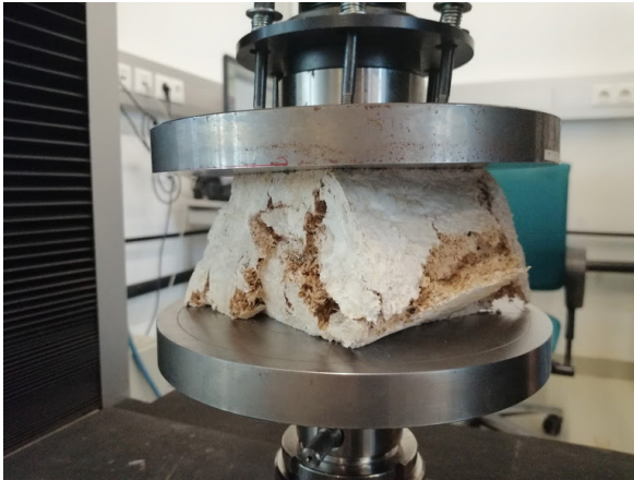
Fig. 104: Unsuccessful compression test
