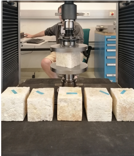
Fig. 108: Beech sawdust samples before testing
