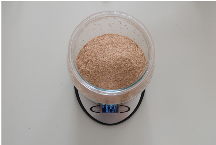
Fig. 60: Weighing the dry substrate
