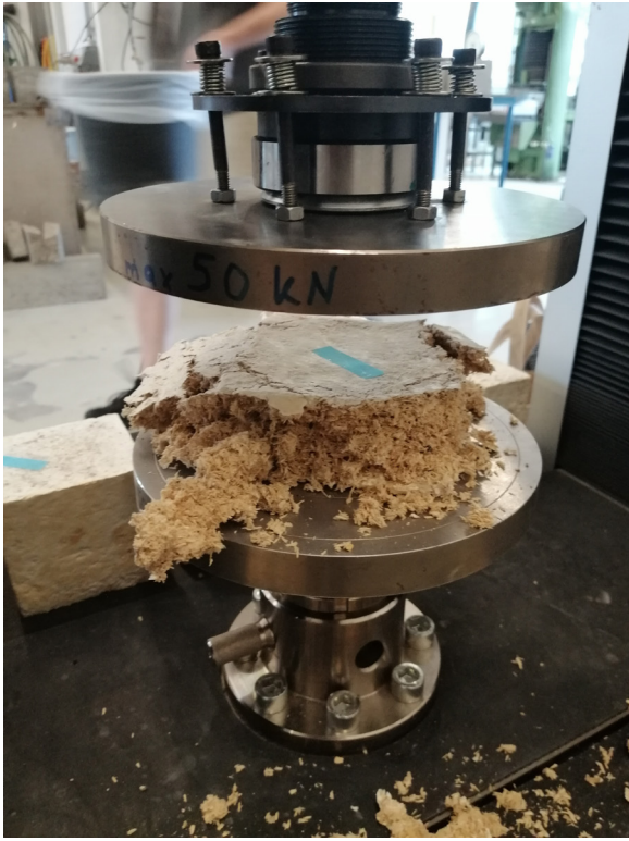
Fig. 123: Compression strength testing - after
