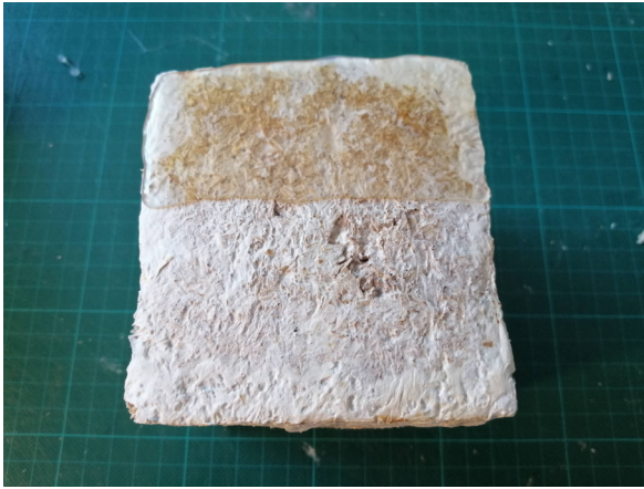
Fig. 138: Sealing the sample surface
