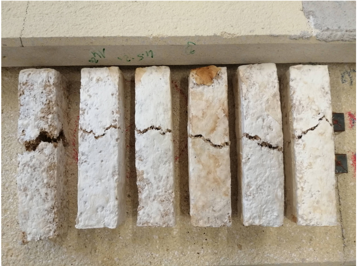
Fig. 125: Beech sawdust samples - after testing
