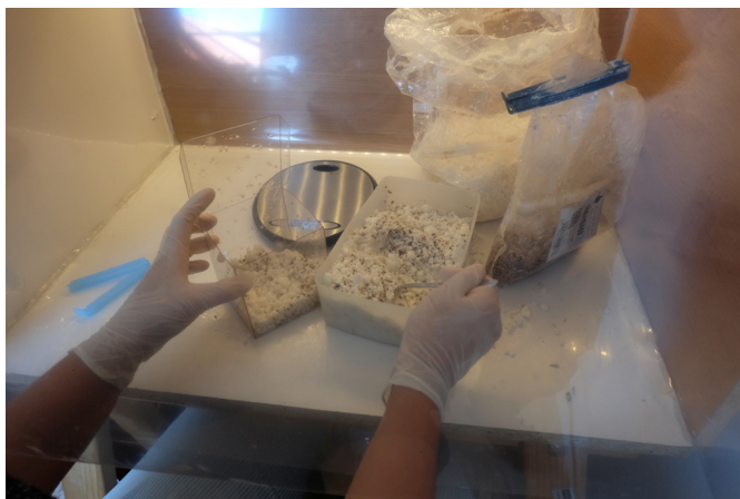
Fig. 63: Filling mould with inoculated mixture
