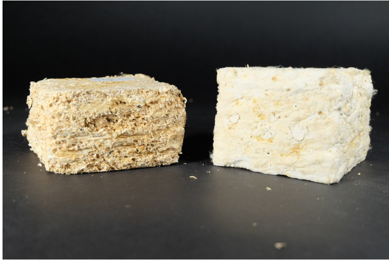
Fig. 117: LM-FSSF-PO-01 and MM-CO-PO-01 - after testing
