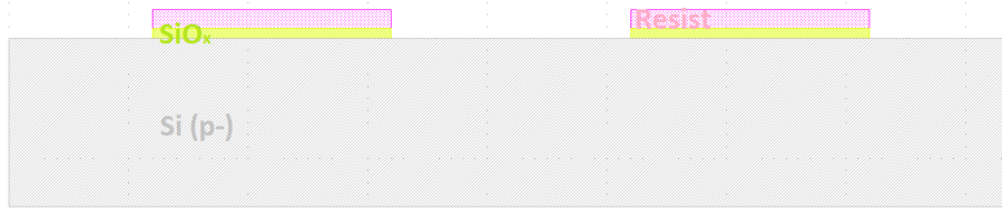
Figure 30: Schematic view of the wafer after structuring of the hardmask.
