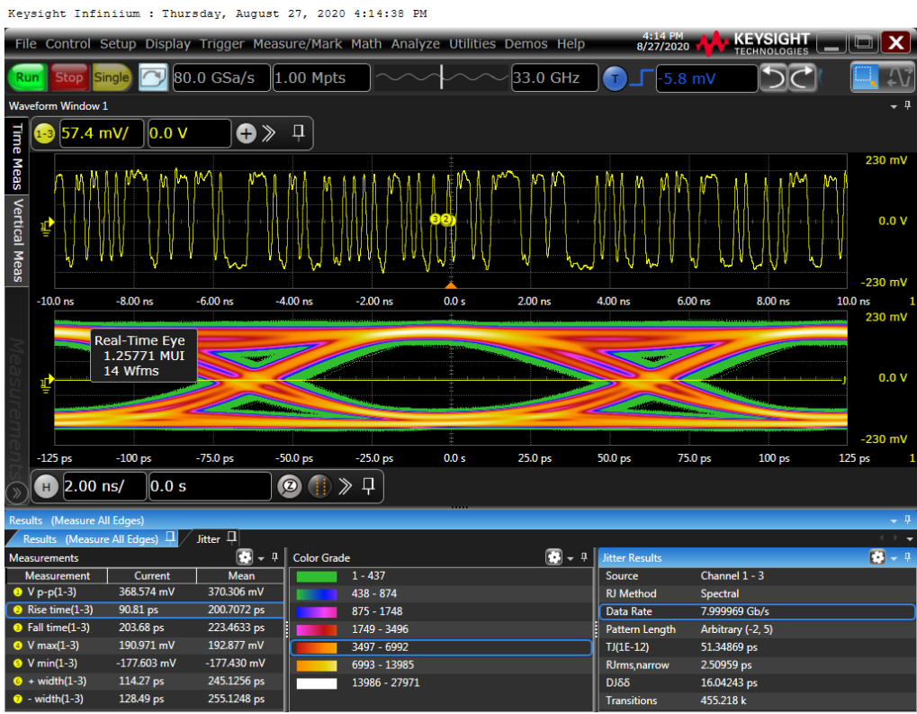
Figure 5.27: Eye Diagram at 8 Gbps
