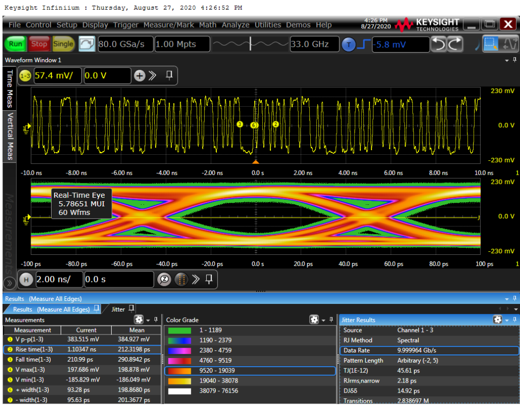
Figure 5.28: Eye Diagram at 10 Gbps
