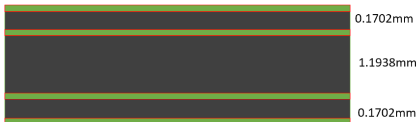
Figure 5.3: Four Layers Stack-up Board of TX and RX. The green parts represent the copper layers, while the gray parts represent the dielectric material.
