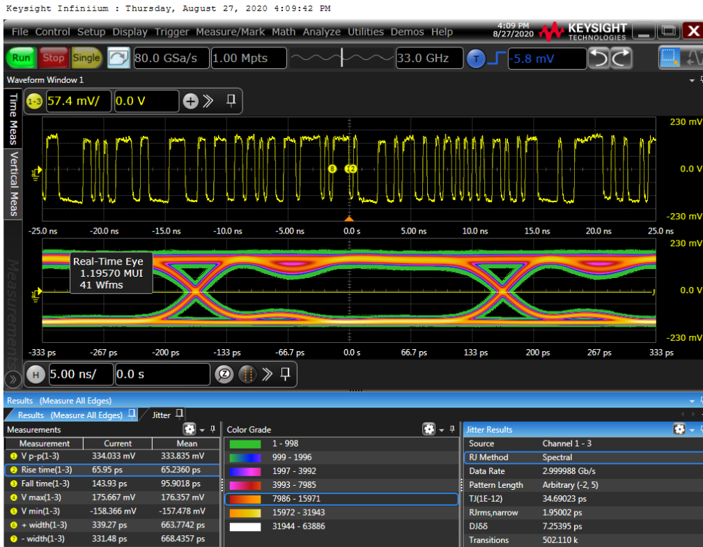
Figure 5.25: Eye Diagram at 3 Gbps
