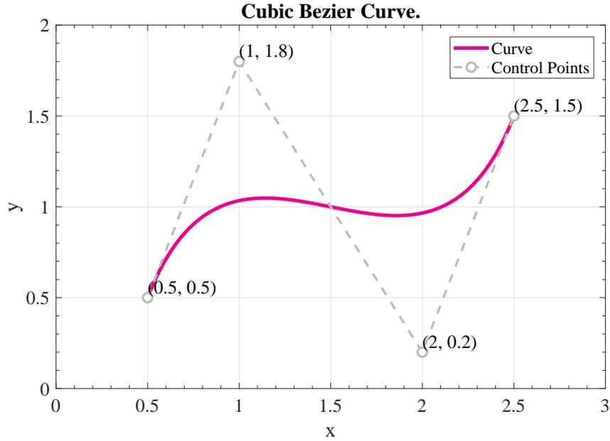
FIGURE A.1: Example of cubic 2D Bezier curve.
