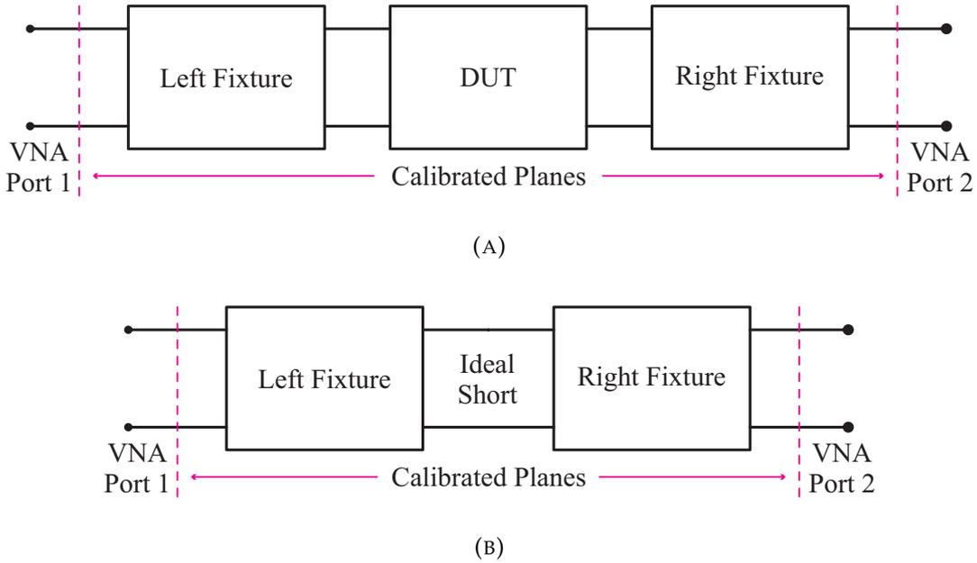
FIGURE 5.3: Illustration of TOD. (A) DUT with left and right fixtures; (B) left and right fixtures connected with an ideal short.
