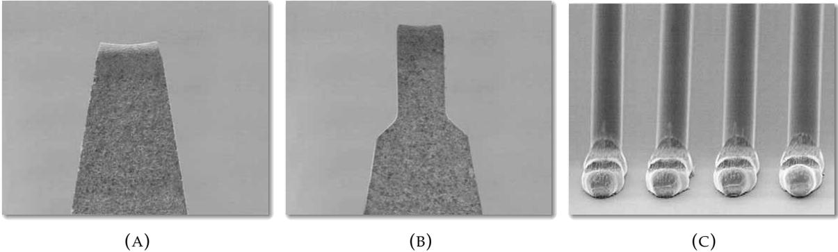
FIGURE 2.9: Standard and fine pitch wedge tools (Source: Micro Point Pro [9]). (A) Standard wedge tool; (B) Fine pitch wedge tool; (C) Fine pitch wirebonds.
