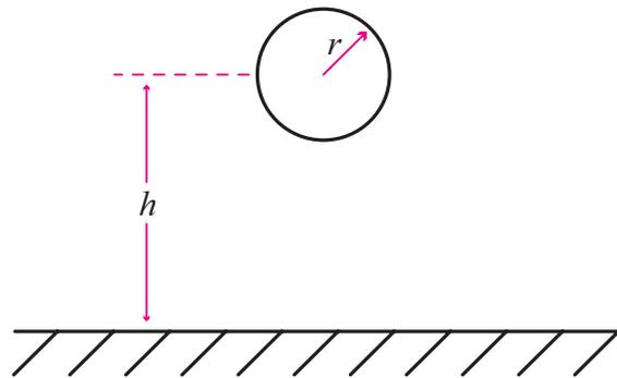
FIGURE 4.12: Capacitance of a wire above a ground plane.
