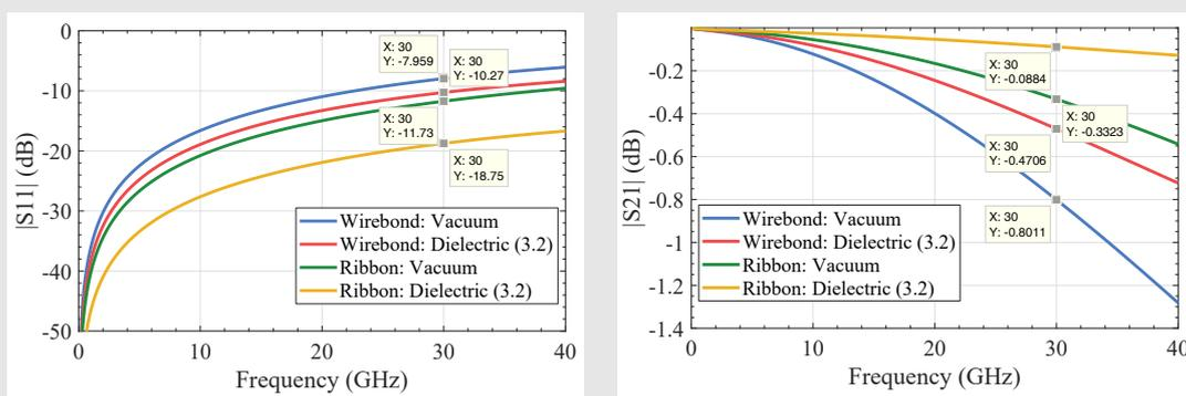
FIGURE 4.22:  $|S_{11}|$  and  $|S_{21}|$  of the simulated structures.
