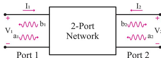
FIGURE 5.1: Illustration of a 2-port network.
