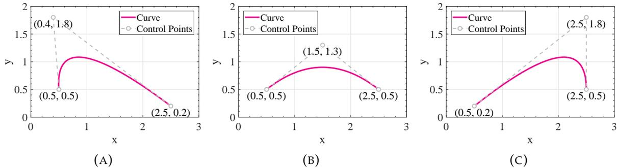
FIGURE 4.14: Illustration of quadratic Bezier curve.
