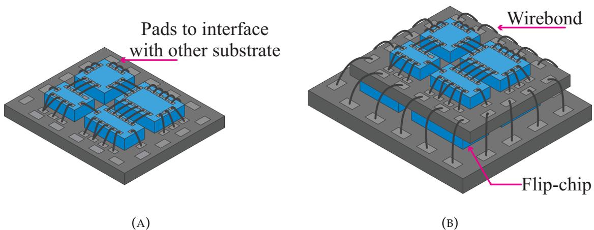
FIGURE 3.2: Illustration of usage of passive silicon interposer.
