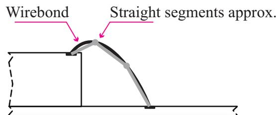
FIGURE 4.9: Illustration of line segmentation of curved wirebonds.
