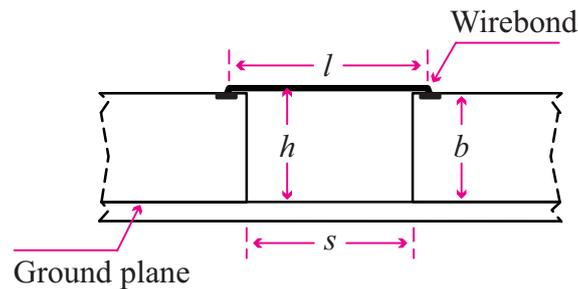
FIGURE 4.6: Straight wirebond over ground.
