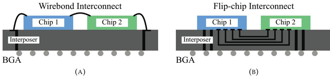
FIGURE 1.1: Illustration of interconnects in 2.5D integration. (A) Wirebond; (B) Flip-chip.
