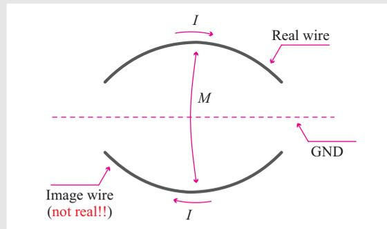
FIGURE 4.16: Image method to estimate effective loop inductance.
