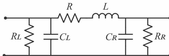
FIGURE 6.17: Bond pads circuit model.
