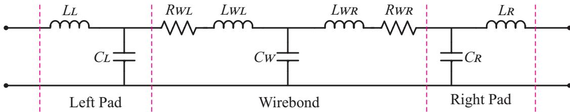
FIGURE 5.6: Grounded wirebond model.
