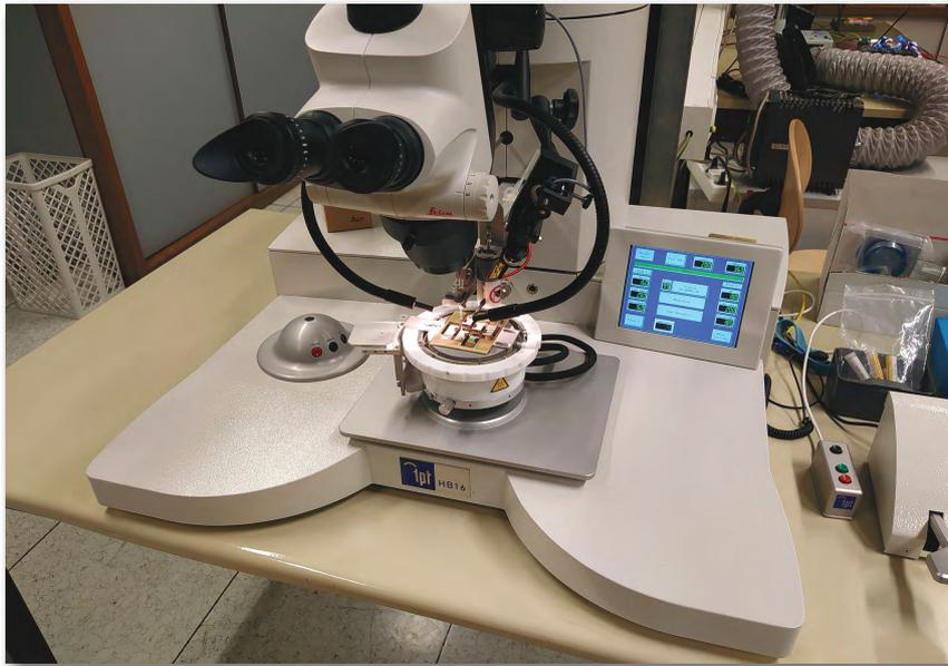
FIGURE 6.3: Bonder machine (TPT-HB16).
