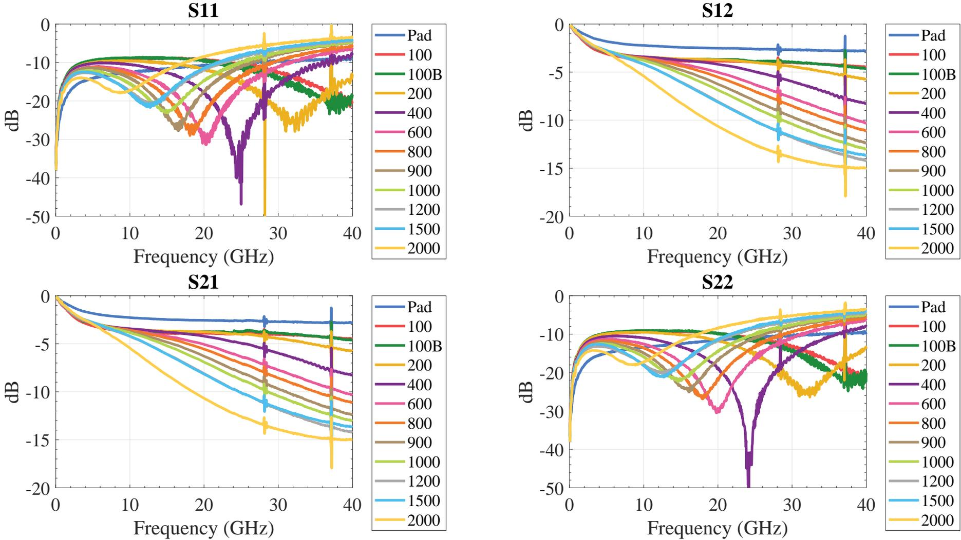
FIGURE 6.9: Wirebonds raw measurements.
