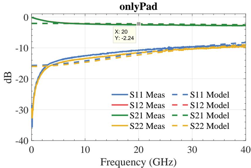
FIGURE 6.18: S-parameter of both circuit model and measurements of the bond pads. Dashed lines represent the model, while solid lines the measurements.
