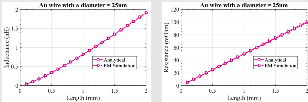
FIGURE 4.5: Inductance and Resistance of straight wire.
