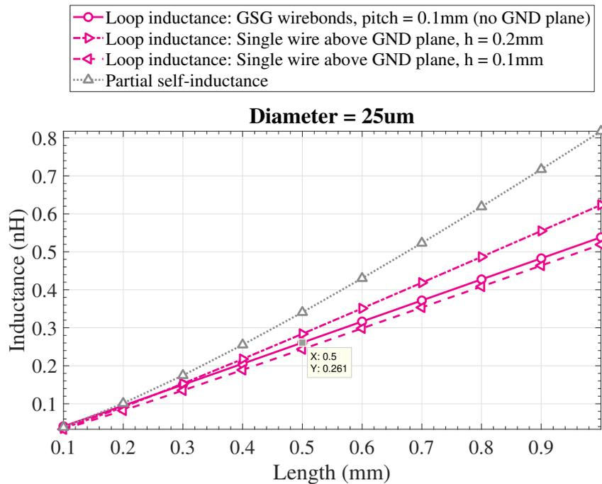
FIGURE 4.24: Inductance of 25  $\mu\text{m}$  wirebond as function of wire length.
