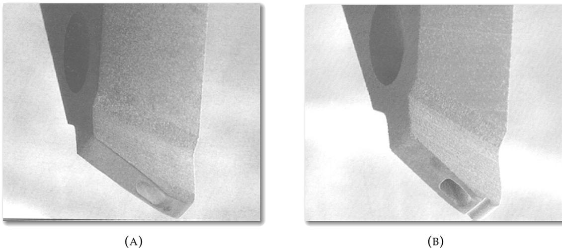
FIGURE 2.3: Wedge tools. (A) for Al wires; (B) for Au wires.
