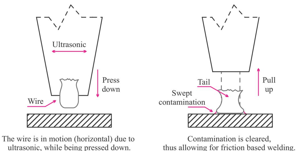
FIGURE 2.2: Ultrasonic bonding process.
