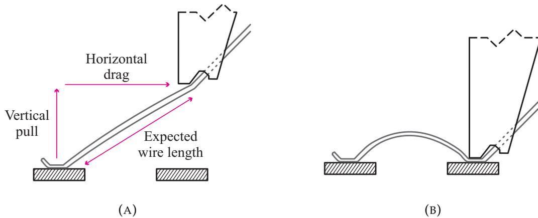
FIGURE 4.15: Simple wedge wire bonding steps.
