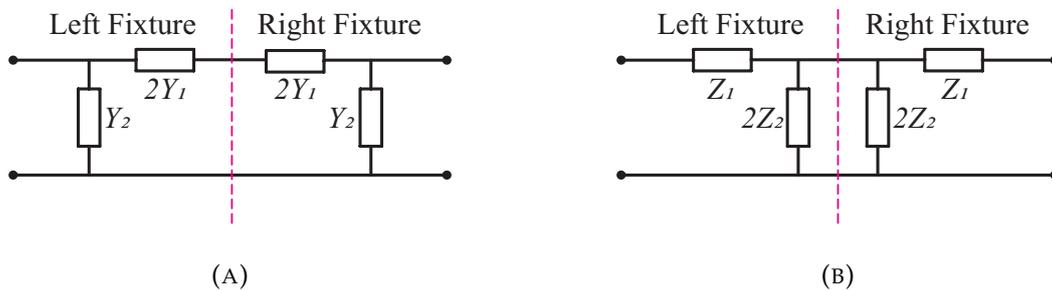
FIGURE 5.4: Bisection of (A)  $\Pi$  and (B) T equivalent circuits.
