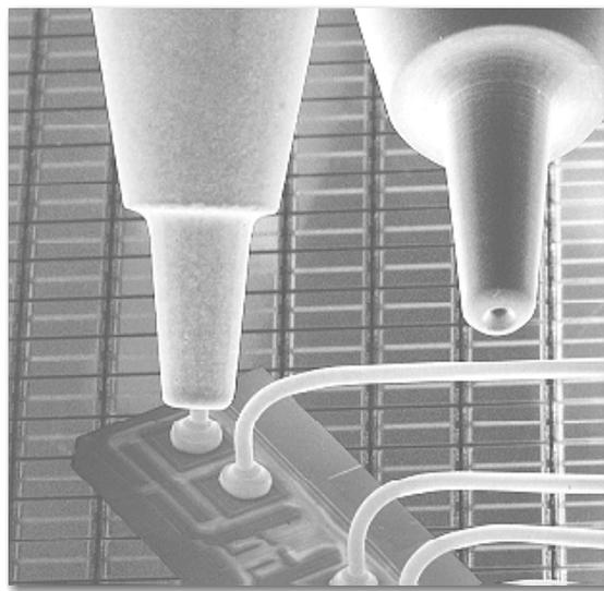
FIGURE 2.5: Capillary for Au ball bonding (after K&amp;S Micro-Swiss [6, Sec. A2.3.2]).
