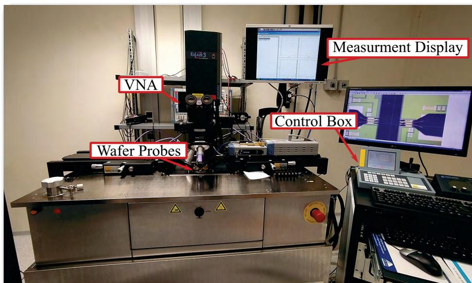
FIGURE 6.5: Wafer probe station.
