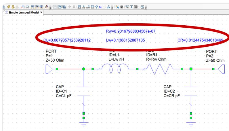
FIGURE 6.13: Schematic and optimization variables in AWR.
