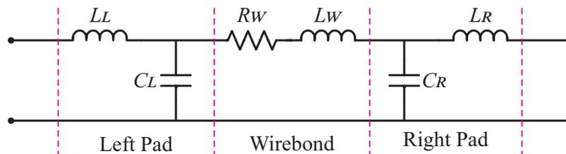
FIGURE 5.5: Non-grounded wirebond model.
