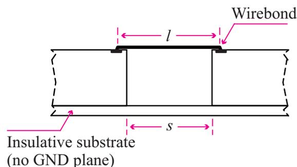
FIGURE 4.3: Illustration of straight wirebond.
