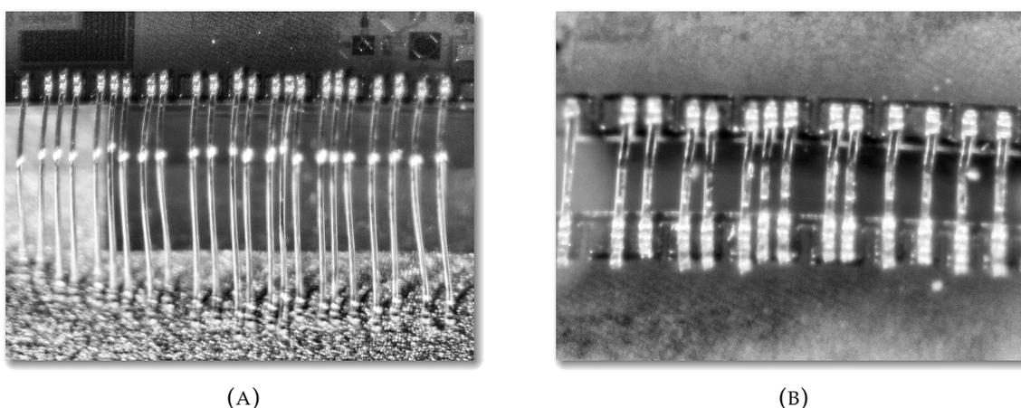
FIGURE 2.1: 25  $\mu\text{m}$  Au wedge wirebonds. (A) Chip-to-substrate; (B) Chip-to-chip.
