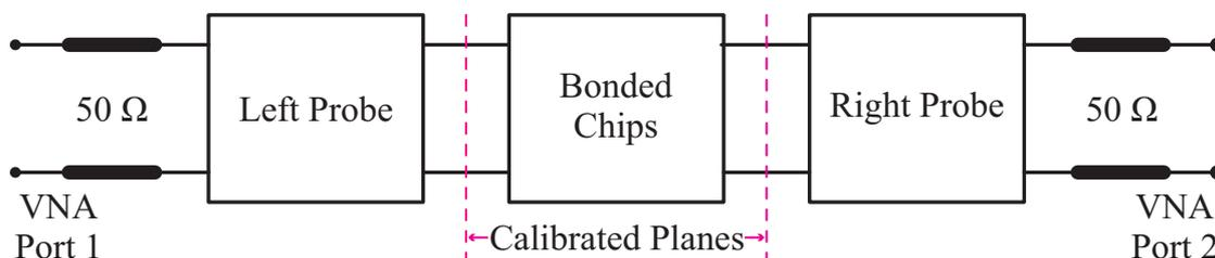
FIGURE 6.1: Block diagram of the measurement setup.
