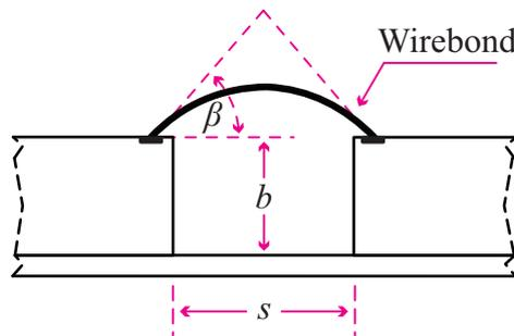
FIGURE 4.13: Curved wirebond modeled as a circle arc.
