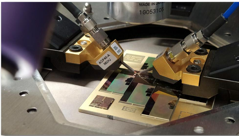
FIGURE 6.4: Wafer probes.
