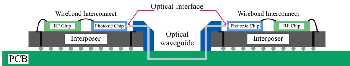
FIGURE 1.2: Illustration of using optical signals to interconnect between heterogeneous integrated systems.
