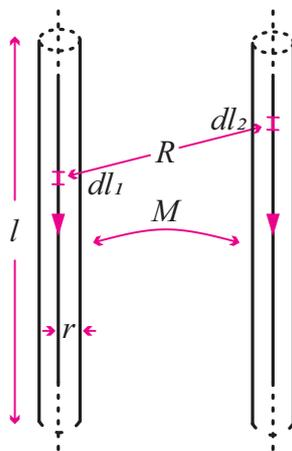
FIGURE 4.10: Illustration of partial mutual inductance of two wires.
