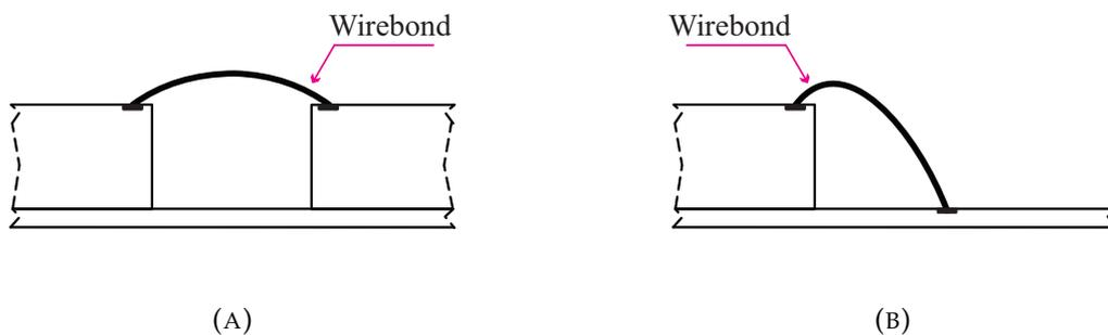
FIGURE 4.7: Illustration of curved wirebonds.
