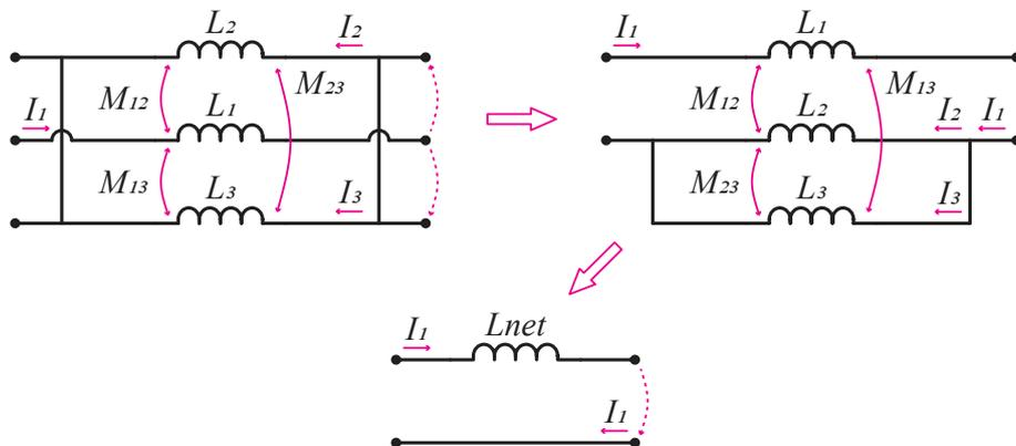
FIGURE 4.23: Equivalent circuit of GSG connected inductors.
