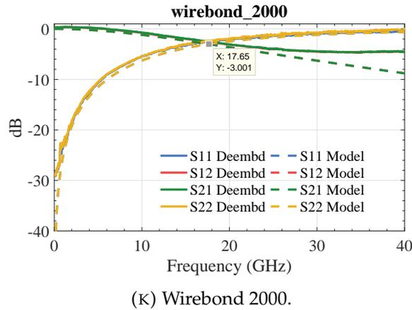
FIGURE 6.20: S-parameters of the de-embedded measurements and the extracted model of the GSG wirebonds.
