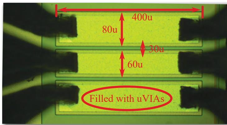
FIGURE 6.6: Measured bond pads.
