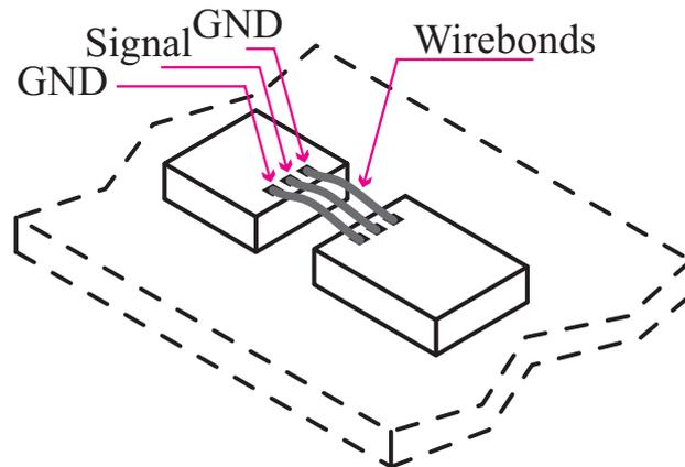
FIGURE 4.19: Illustration of GSG wirebonds.
