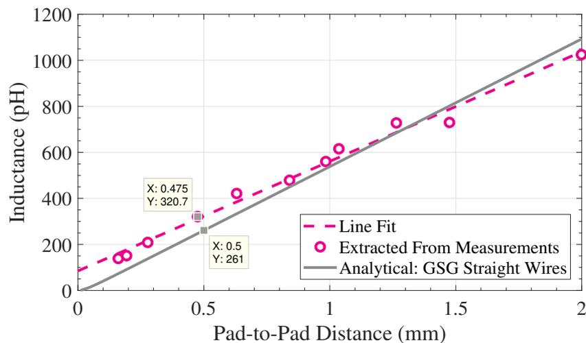
FIGURE 6.21: Extracted inductance as a function of pad-to-pad distance.
