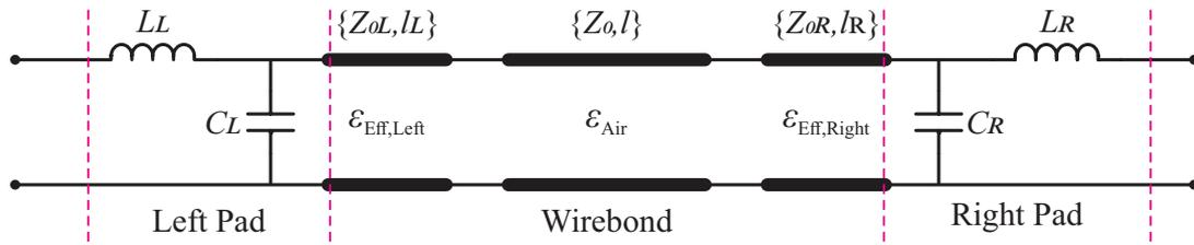
FIGURE 5.8: Wirebond modeled as multi-segmented transmission line.
