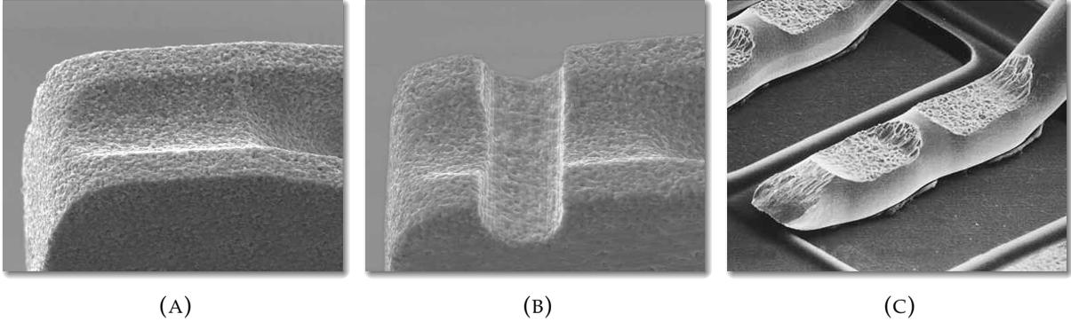
FIGURE 2.10: Reducing deformation width of wirebonds by incorporating a linear groove in wedge tools (Source: Micro Point Pro [9]). (A) Linear grooved wedge tool for Al bonding; (B) Linear and cross grooved wedge tool for Au bonding; (C) Au wirebond with linear and cross groove wedge tool.
