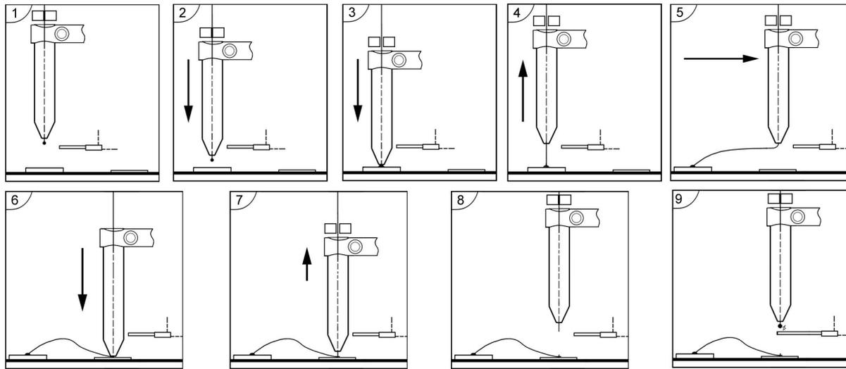
FIGURE 2.6: Thermosonic Au ball bonding (Source: TPT [5]).
