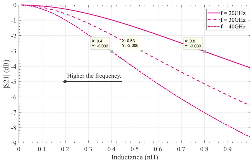
FIGURE 2.7: Transmission coefficient of a series inductance.
