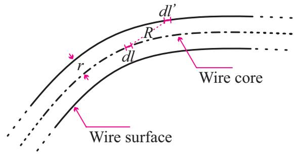
FIGURE 4.11: Neumann partial self-inductance of a wire.
