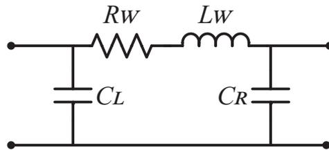
FIGURE 4.8: Simplified lumped model for curved wirebond.
