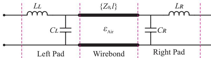
FIGURE 5.7: Wirebond modeled as one section transmission line.
