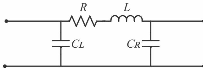
FIGURE 6.19: Wirebonds circuit model.
