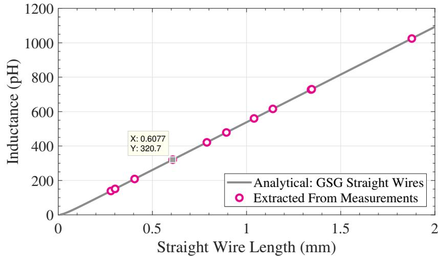
FIGURE 6.22: Expected straight wire length from the extracted inductance values.
