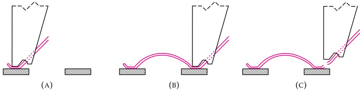
FIGURE 2.4: Wedge bonding process.
