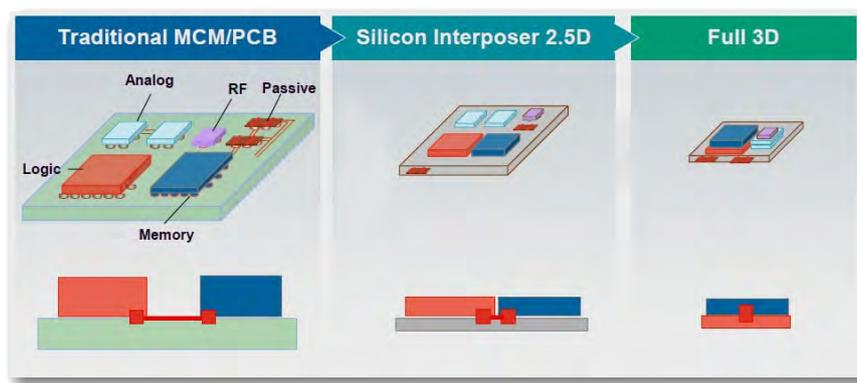
FIGURE 3.1: Evolution of chip integration (Source: Adapted from [10]).
