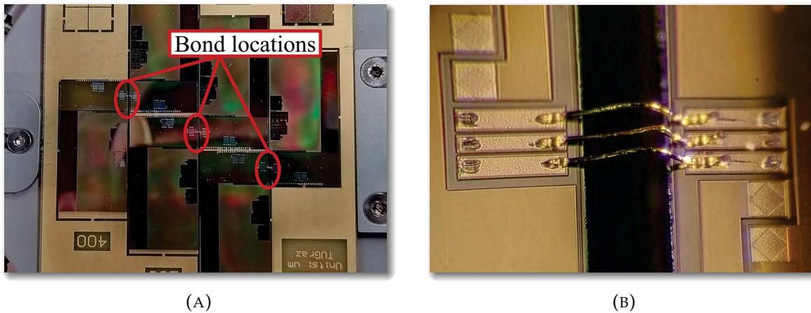
FIGURE 6.2: Photo of bonded interposer chips. (A) Interposers glued on a carrier PCB. (B) A zoomed photo of the GSG wirebonds (“Wirebond 400”).
