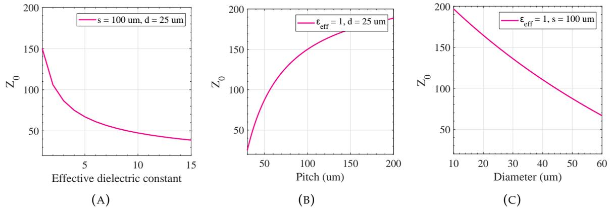
FIGURE 4.20: Characteristic impedance of GSG wirebonds. (A) Varying  $\epsilon_{eff}$ , (B) Varying pitch distance, (C) Varying wire diameter.
