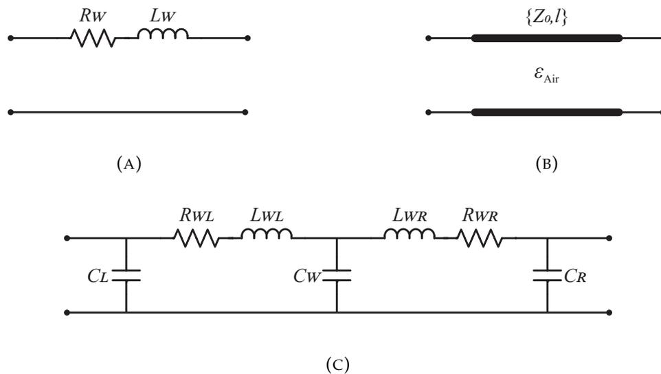
FIGURE 4.2: Equivalent circuit model of wirebonds. (A) A simple lumped model when parasitic capacitance is negligible. (B) Transmission line (typically lossless) model when wirebonds have uniform geometry around a ground net (e.g., coplanar structure). (C) A more complex lumped model to account for capacitance.
