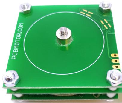
Figure 3.6.: PCB piezo motor: 30 mm motor with 200 step encoder, position sensor and controller - modified from "www.pcbmotor.com"; last accessed 03.08.2020.
