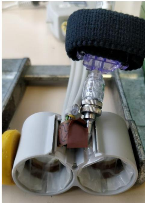
Figure 3.1.: Adapted cuff for the fluid system with connected pressure sensor (black strap).
