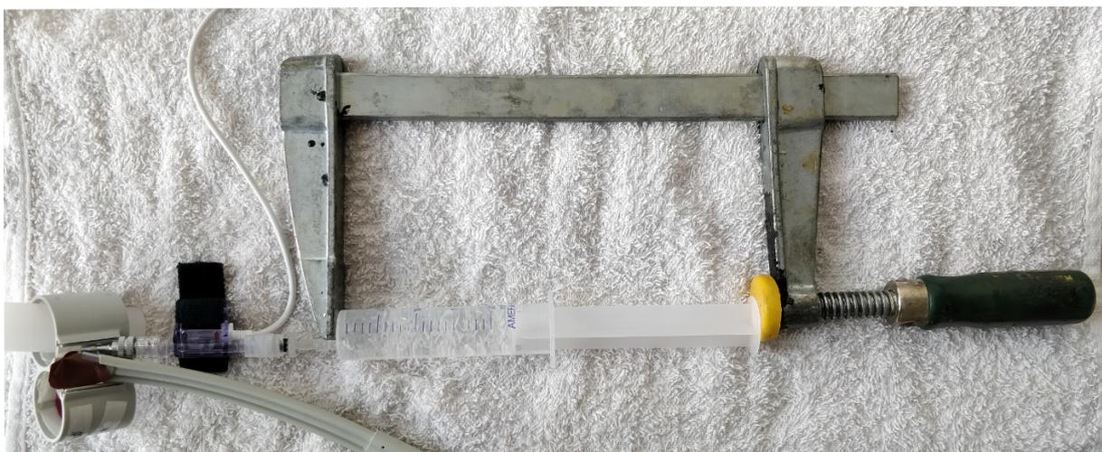
Figure 3.2.: Prototype V.0: Mechanical actuator - syringe - pressure sensor - cuff. Suitability test of the selected approach.
