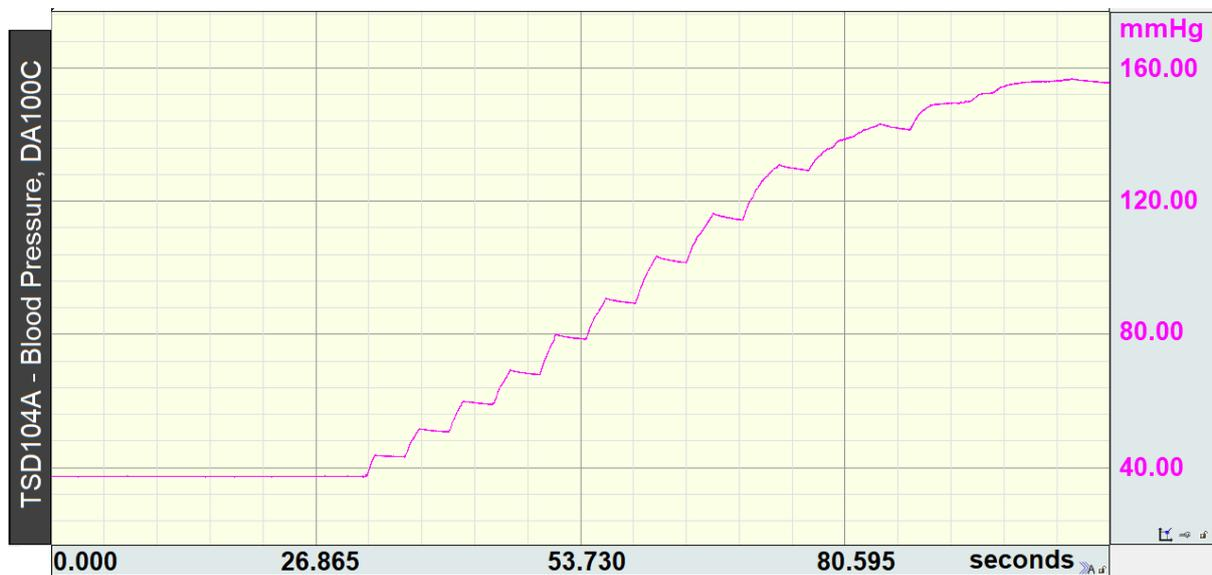
Figure 4.14.: Prototype V.3. First setup. Control with 11 x 100 steps, between the 100 steps 3 seconds stop. Pressure increase of 38 to 158 mmHg
