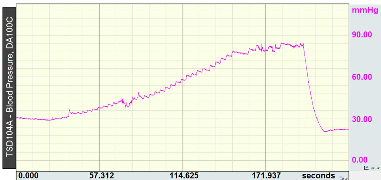
Figure 4.19.: Prototype V.3. Third setup. Control with 30 x 50 steps (increase to 34 x 50 until motor stalling), between the 50 steps 3 seconds stop. Pressure increase from 30 to 80 mmHg.
