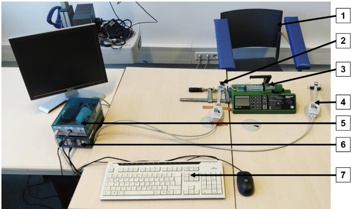
Figure 3.5.: Measurement setup for the comparative measurement of CNAP2GO (prototype V.2) and the CNAP classic system with aforementioned COVID-19 safety measures.
