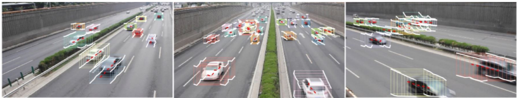
Figure 2.21: Spatial-temporal bounding tubes to model the vehicle's motion [51]
