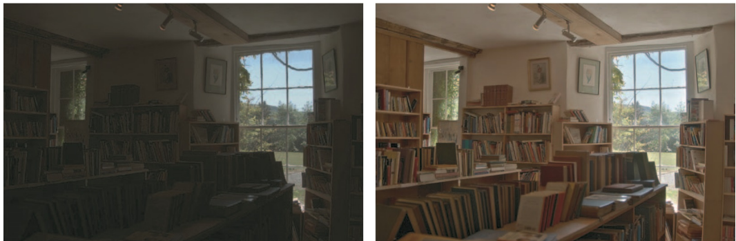
Figure 2.3: HDR image: Linear scaling versus tone-mapped result [75]
