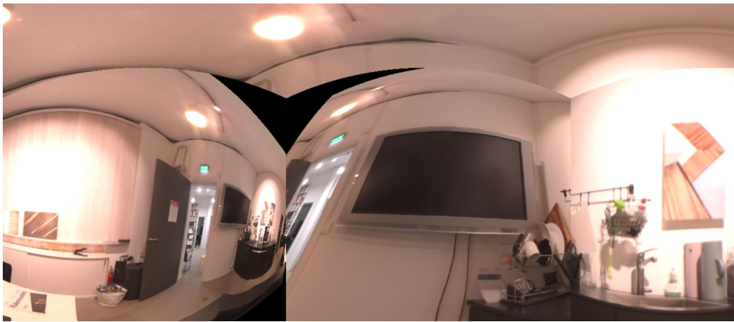
(b) Warping errors: duplicate objects, distortions and holes
