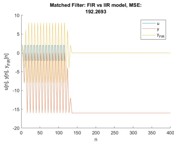
Figure 3.12: System errors due to rounding inside filter structure.
