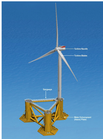
Figure 3.4: Prototype schematic [18]. Figure 3.5: WindFloat prototype [18].
