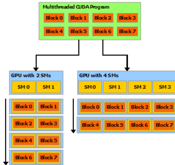
Figure 1.3.: Illustration of the distribution of blocks to Streaming Multiprocessors. While the programmer can choose the number of blocks, the number of Streaming Multiprocessors only depends on the GPU. A GPU with more multiprocessors will automatically execute the program faster. Reprinted from “CUDA C Programming Guide” by NVIDIA Corporation. Copyright 2007-2020 by NVIDIA Corporation.
