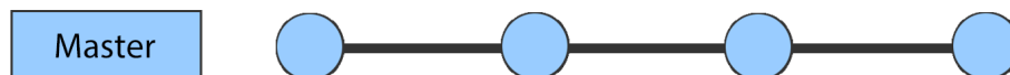
Figure 5.1: Single branch Git workflow: A basic Git workflow is using a single branch, typically called the master branch. In this example, the master branch consists of four consecutive commits. Each commit represents a snapshot of the project.
