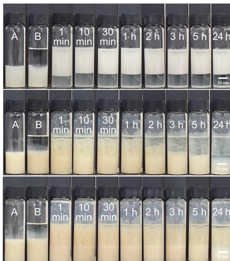
Figure B-4: Photos of vessels containing cyclohexane-in-water emulsions stabilized by particles of \text{Ce}_{0.495}\text{Sn}_{0.495}\text{Pd}_{0.01}\text{O}_{2-\delta} at concentrations in water of 0.03 wt% (upper), 0.30 wt% (middle) and 1.0 wt% (lower) at different times since preparation. A is the aqueous dispersion of particles, B is after addition of oil but before emulsification.
