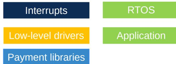
Figure 1.2: Software components of a payment terminal
